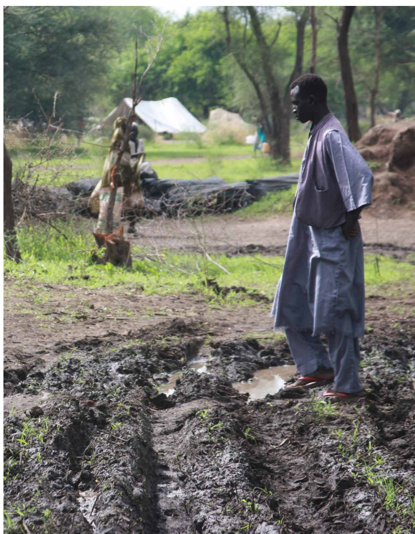
Black cotton soil with the rain makes roads and airstrips unusable. Photo credit: European Commission DG ECHO/Flickr.com/CC BY-SA 2.0
