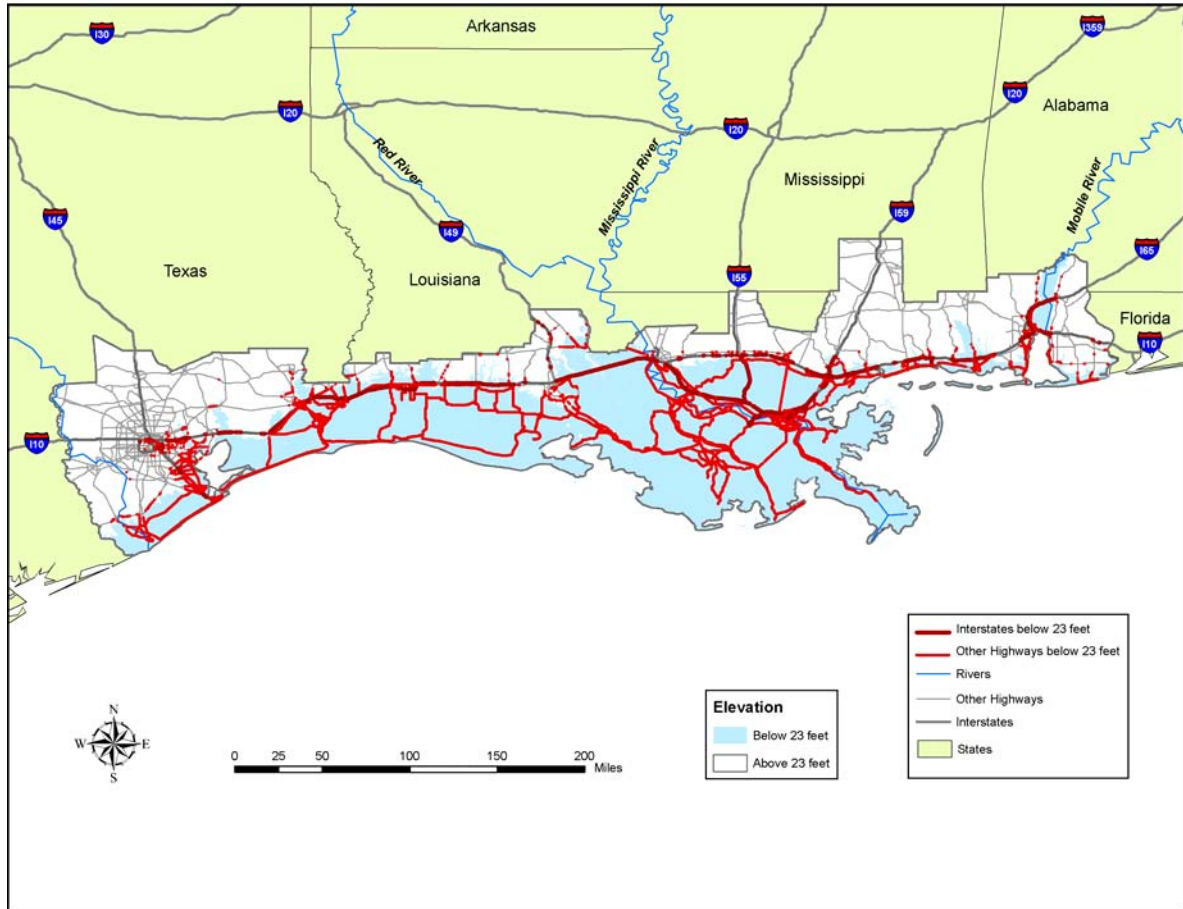
Figure 4.6 Highways currently at risk from storm surge at elevations currently below 7.0 m (23 ft). (Source: Cambridge Systematics analysis of U.S. DOT data)
