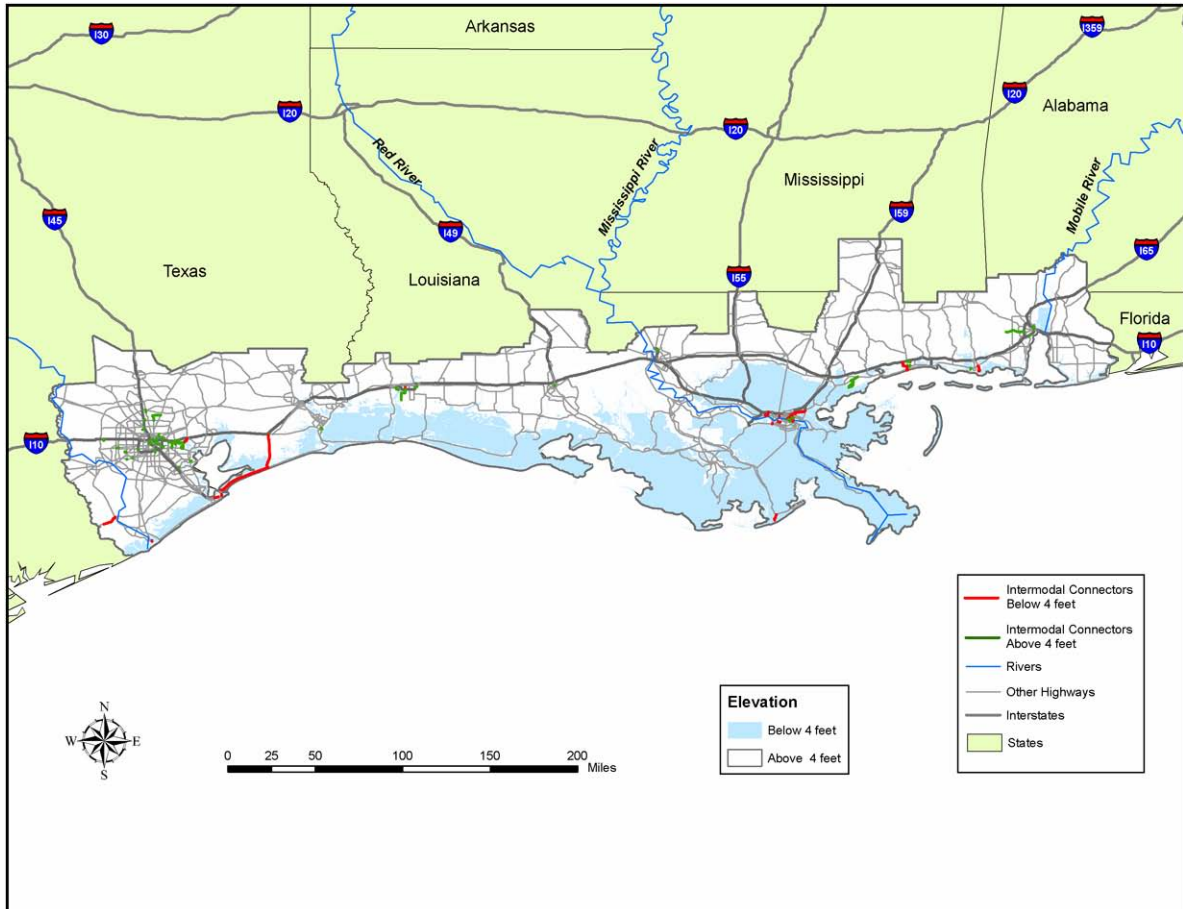
Figure 4.3 National Highway System (NHS) intermodal connectors at risk from a relative sea level rise of 122 cm (4 ft). (Source: Cambridge Systematics analysis of U.S. DOT data)
