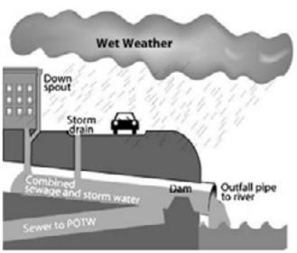
**Figure 2.** Under normal conditions, a combined sewer system distributes all sewage to a treatment plant. Heavy rainfall can cause overflows, sending some untreated sewage into nearby waterways. Credit: EPA.
