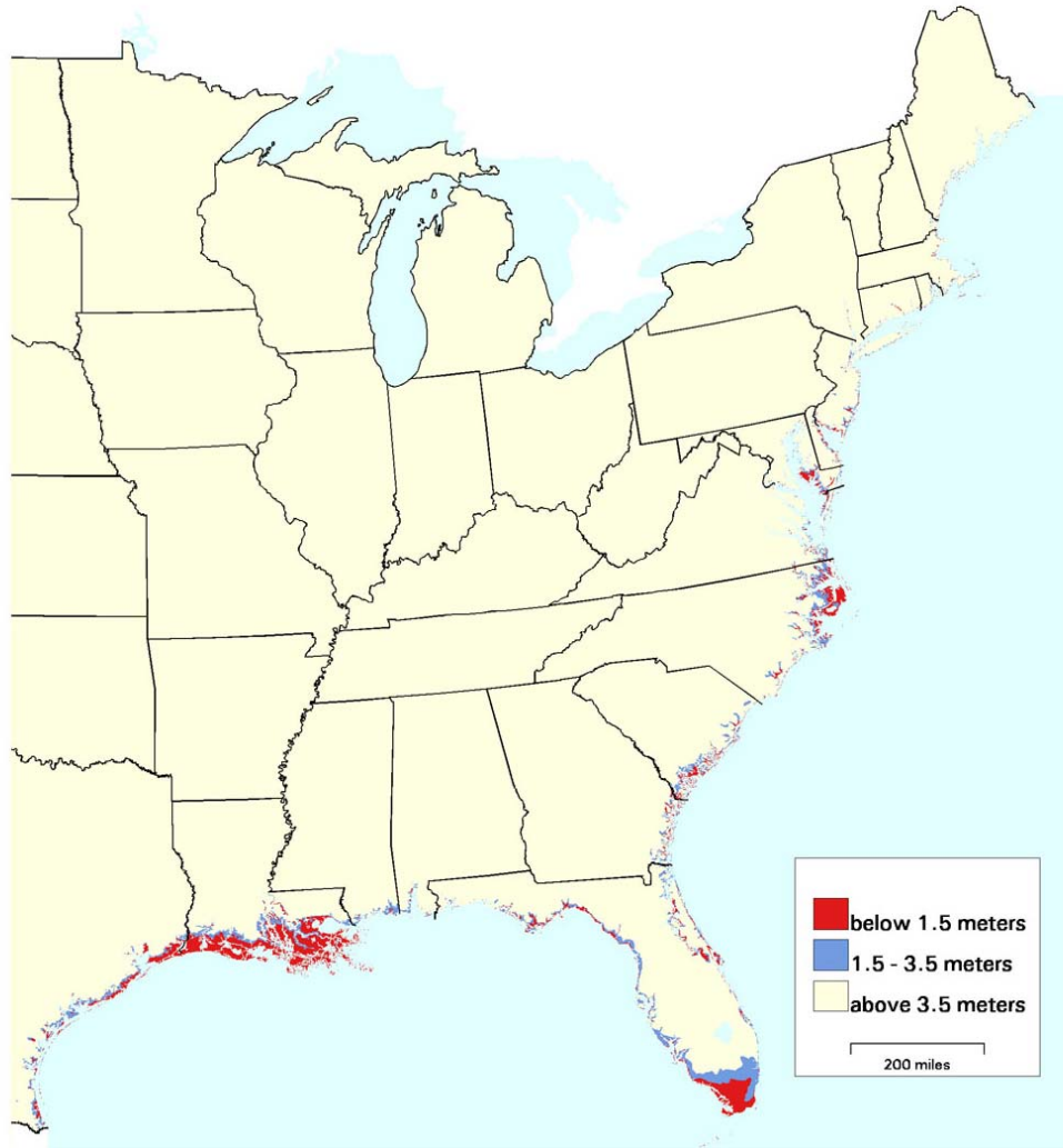
Figure 2. Map of lands close to sea level along the U.S. Atlantic and Gulf Coasts. Although the results nominally are in meters, the 1.5 meter contour is primarily based on the 5-ft NGVD contour from USGS topographic maps. Source: Titus and Richman (2001). 6
