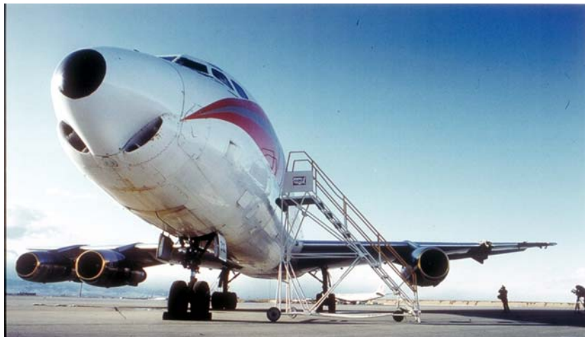
Figure 3. Photo of an aircraft missing an engine which had been torn off by turbulence.
