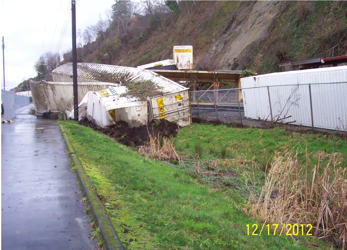
Figure 3. Terminal Avenue train car derailed by landslide (photograph courtesy of Port of Everett).
