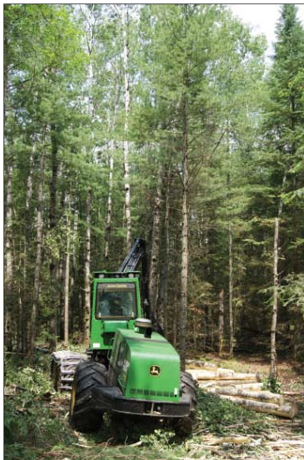
Working carefully around a crop tree during a white pine thinning operation with cut-to-length harvesting equipment. Photo by John Rajala, Rajala Companies, used with permission.
