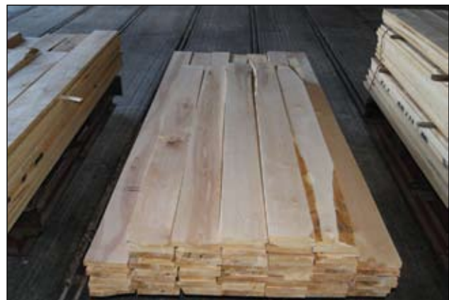
Kiln-dried paper birch lumber with discolored heartwood. Stress leads to discoloration of the heartwood, lowering the value of the lumber. Photo by John Rajala, Rajala Companies, used with permission.
