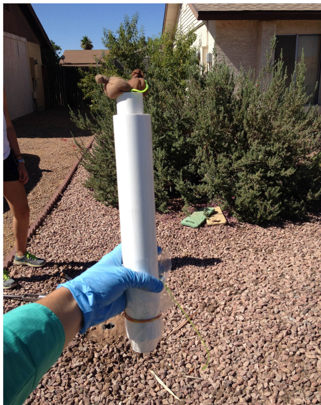
Figure A1. The 30 cm depth resins were installed using a double-PVC pipe apparatus. The outside larger pipe was permanently installed at an angle in the soil during the study. The smaller, inner pipe, was used to hold and replace the resins. The resins sat at the bottom end of the tube (shown here upside down) and the opposite end was capped using plastic sheeting to prevent any precipitation or irrigation water reaching the resin bags that did not first travel through the soil column.
