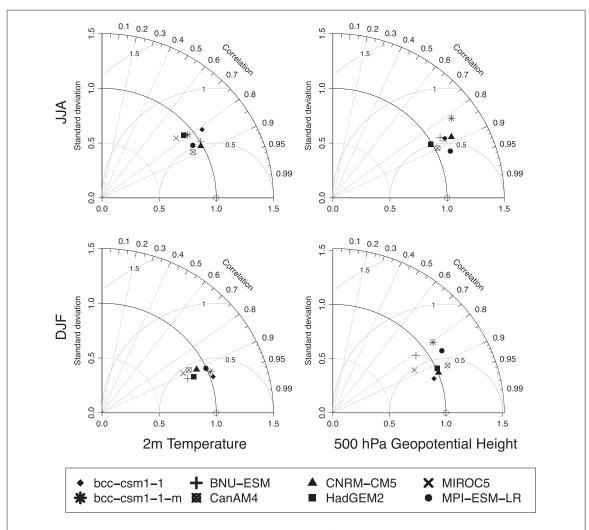
**Figure 6.** Taylor diagrams of the models used in this study for composites of the near-surface temperature (left) and 500 hPa geopotential height (right) for hot summer (upper row) and cold winter (lower row) events over Central Europe.
