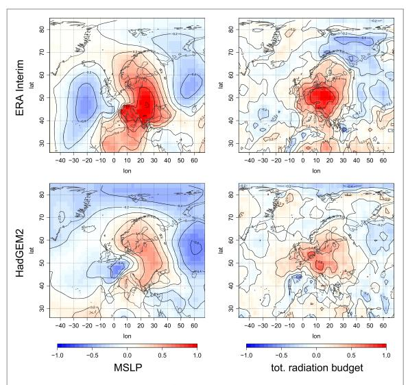
Figure 5. JJA. Composites of the standardized MSLP (left) and total radiation budget (right) for warm summer events in ERA interim (upper row) and HadGEM2-A (lower row). Note that positive values in the total radiation budget denote radiative heating of the surface. Values outside of  $\pm 0.18$  are significantly different from 0 at 0.05 significance (determined through a student's t-test).
