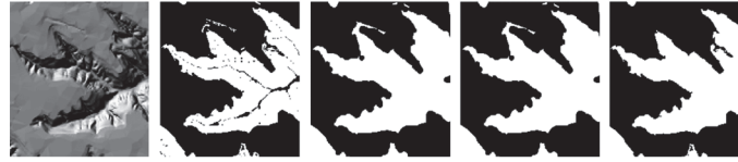
Fig 3. A terrain mask by different morphological method. (a) hillshade image of DEM; (b) terrain mask by Jenks natural breaks only; (c) mask after opening operation; (d) mask after closing operation; (e) mask after reconstruction.
