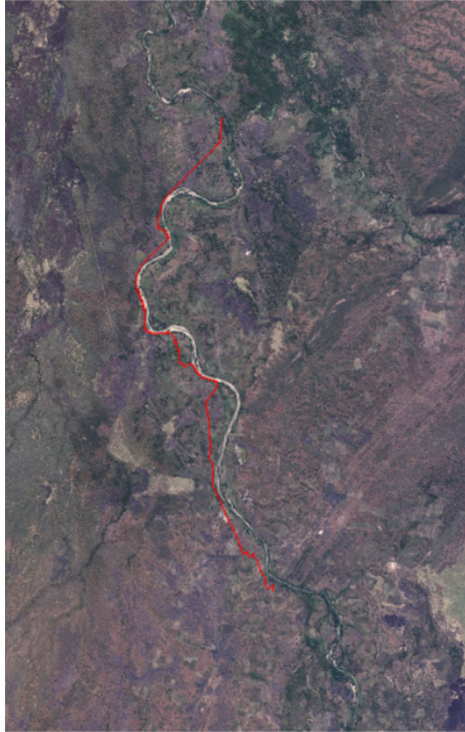
Fig 4. Example path produced using the A* and land classification between arbitrary points. Arbitrary points were used to emphasise how the algorithm diverts the path around a prominent obstacle; in this case, the river itself (Produced using Bing aerial imagery).
