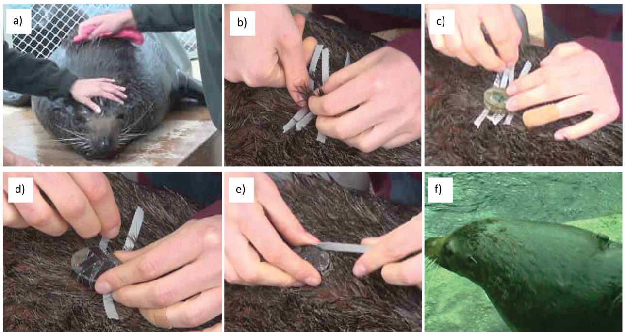
Fig 1. Process of accelerometer attachment with tape. a) Dry the fur; b) Lift the hair to stick tape to undercoat; c-e) Tape on the accelerometer; f) Seal with accelerometer.
