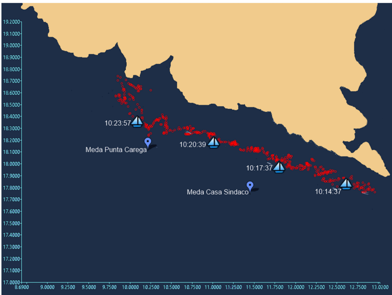
Fig 16. Boat tracking event recorded on March, 23rd 2015. The panel shows a 5 km route of a passenger vessel moving in the study area. The red circles correspond to the position of the boat every 1 second, as reconstructed by the PAM system. The boat-shaped placemarks correspond to the AIS-recorded position of the boat. The good correspondence confirms the efficiency of the boat tracking algorithm.
