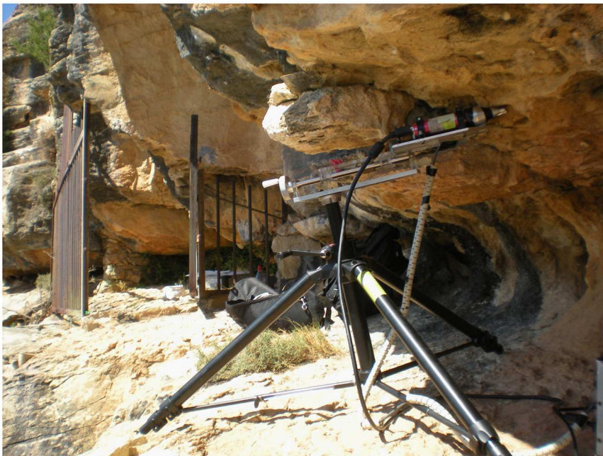
Fig 4. Portable EDXRF spectrometer used in Les Dogues.
