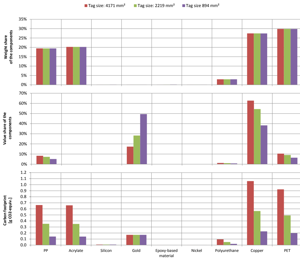
Figure 11. RFID tags with Cu aerials and PP faces
