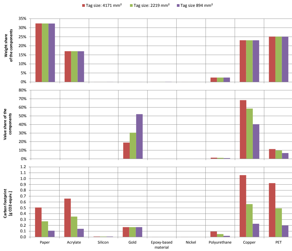
Figure 10. RFID tags with Cu aeriels and paper faces
