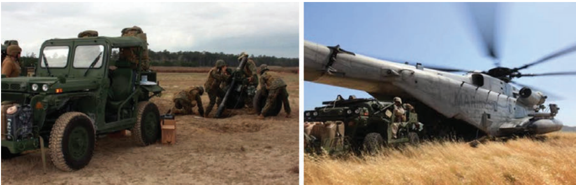
Figure 3.13 USMC Internally Transportable Vehicle (ITV) Delivered by CH-53 (left) to Carry and Support 120-mm Mortars (right)
