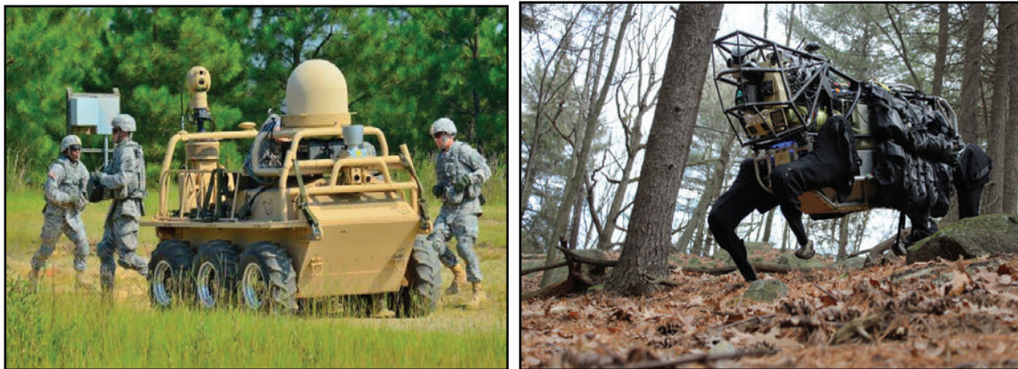
Figure 3.10 Unmanned UTM Prototypes: Lockheed Martin Robotic Mule (left), and DARPA Legged Squad Support System (LS3) (right)
