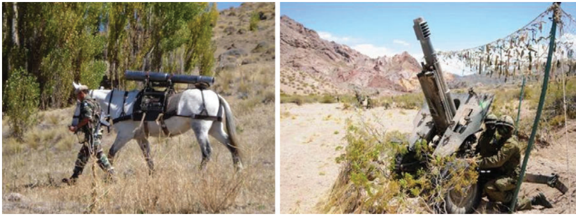
Figure A.13 Argentinian Army Mule Packing a Howitzer Barrel (left) for the OTO Melara Mod-56 105-mm Mountain Howitzer (right)
