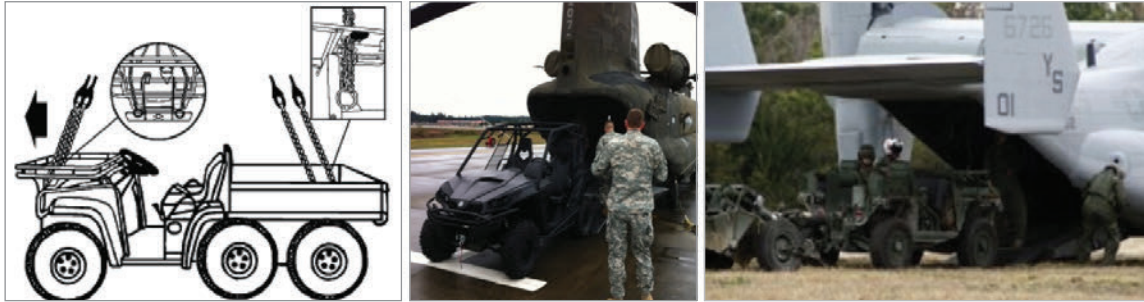
Figure 4.9 Internal and External Transport of UTM Platforms by Rotary-Wing and VTOL Aircraft
