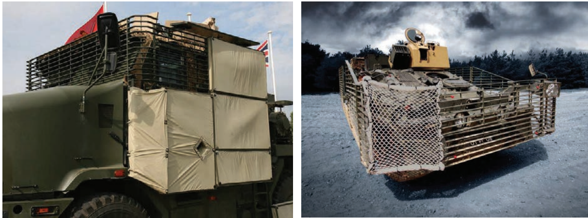
Figure 5.1. Tarian Protective Fabric on the British HET (left) and Spartan (right) Vehicles
