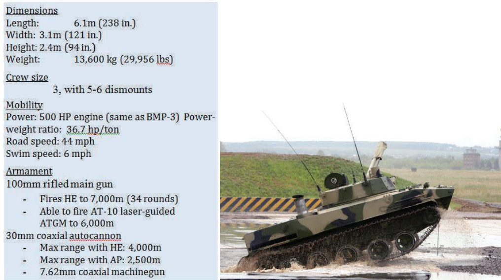
Figure 2.4. Russia's BMD-4M—Technical Specifications
