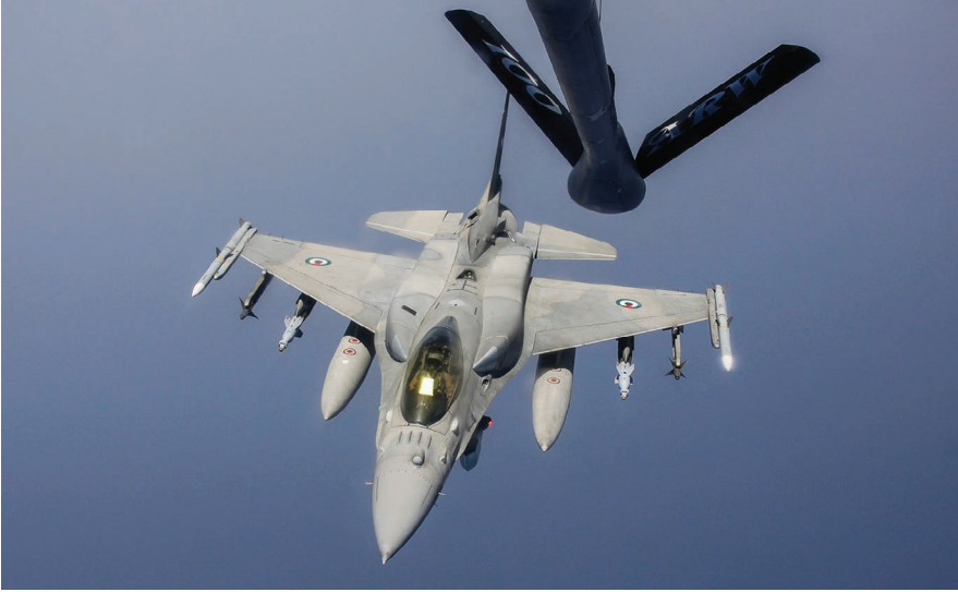
A UAE Air Force F-16E Desert Falcon breaks away after refueling from a UK-based USAF KC-135R Stratotanker of the 100th Air Refueling Wing over the Mediterranean on July 19, 2011. Inbound to Libya, the fighter's armament comprises AIM-102C and AIM-9M air-to-air missiles, GBU-24 Paveway III laser-guided bombs, and an AN/AAQ-32 Internal FLIR Targeting System pod.
