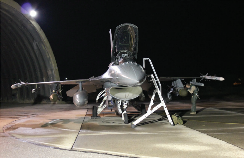
A Norwegian fighter pilot performing a final check of his F-16AM shortly before take-off from Souda Air Base, Crete. In addition to AIM-120B AMRAAM missiles, the aircraft is armed with GBU-31(V)1/B and GBU-31(V)3/B PGMs, the latter designed to penetrate hard targets such as bunkers.
