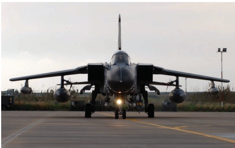
AMI Tornado ECR at Trapani, Air Base, Sicily, carrying HARM anti-radiation missiles on its fuselage hardpoints for a SEAD mission.
