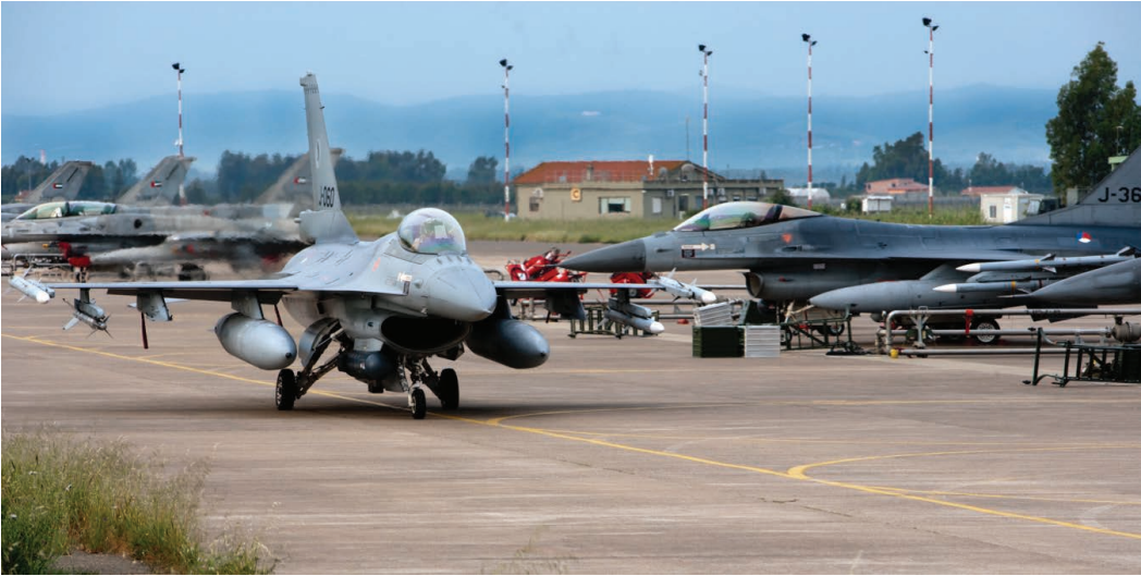
Royal Netherlands Air Force F-16AM taxiing at Decimomannu Air Base, Sardinia, on April 21, 2011. It carries the standard Dutch armament for OUP comprising one short-range AIM-9L and three medium-range AIM-120B AMRAAM air-to-air missiles. All RNLAF F-16s flying missions over Libya were equipped with the Litening Advanced Targeting Pod (ATP), enabling them to conduct so-called non-traditional ISR missions. In the background are UAE F-16E/Fs.
