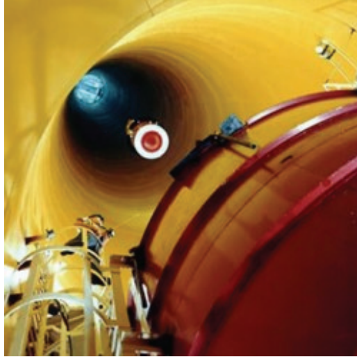
NASA drop tower. View of free fall in vacuum chamber
