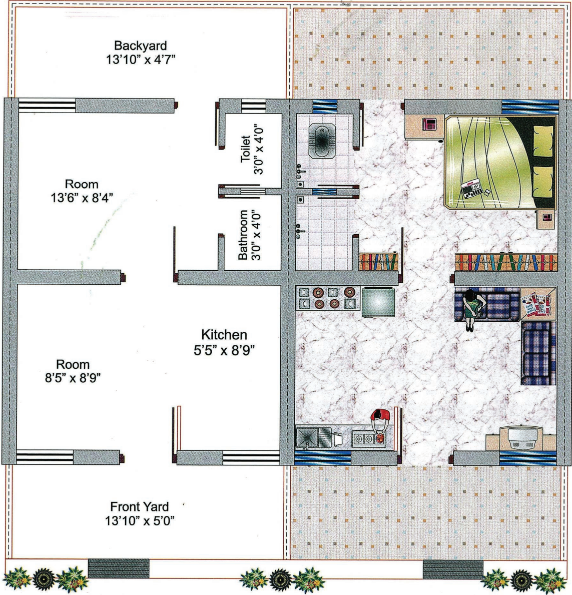
Figure A.2 Ashray Housing-Unit Floor Plan: Two Bedroom with Hall and Kitchen
