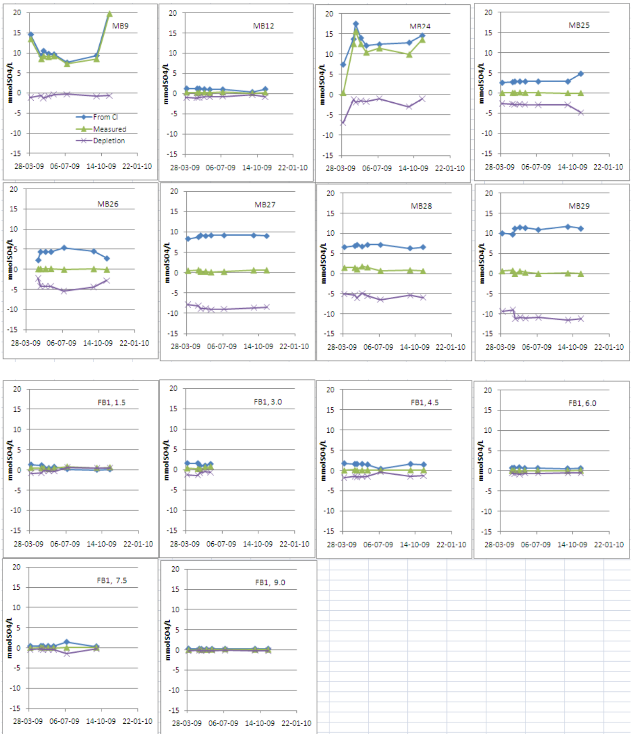
Figure 8: Temporal variation in 14 dipwells/piezometers in the sulphate concentration measured [SO_4^{2-}] , along with the theoretical concentration ( 0.052 * [Cl] ) and the sulphate depletion ( [SO_4^{2-}] - 0.052 * [Cl] ), where 0.052 is the SO_4:Cl ratio normally found in seawater.
