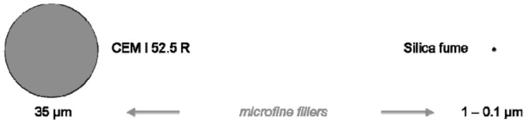
Figure 10 To fill the voids between the cement particles, a larger amount of silica fume is needed [34]
