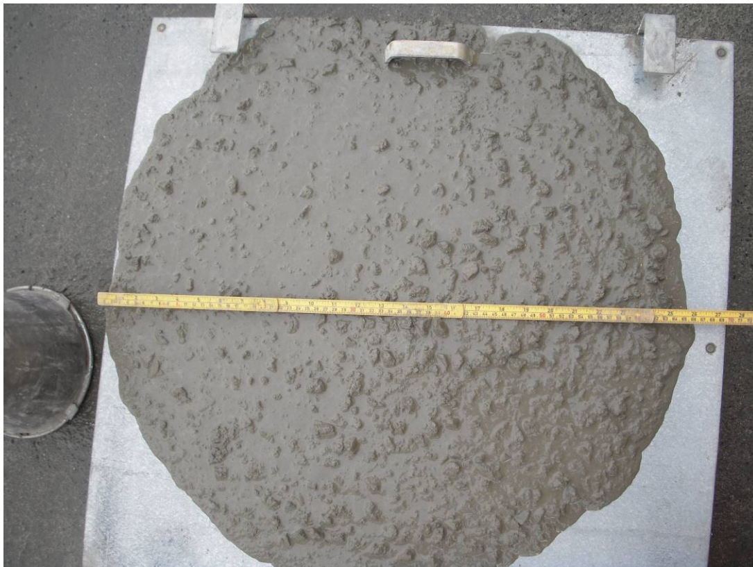
Figure 3-21 Grading R1-42 at a matrix volume of 444 l/m 3 (w/c=0.57) and slump-flow of 650 mm
