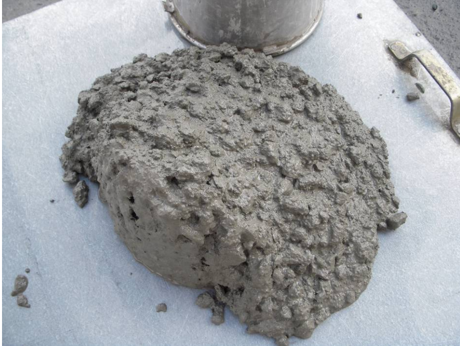
Figure 3-16 Grading R1-32 at a matrix volume of 395 \text{ l/m}^3 ( w/c=0.57 )
