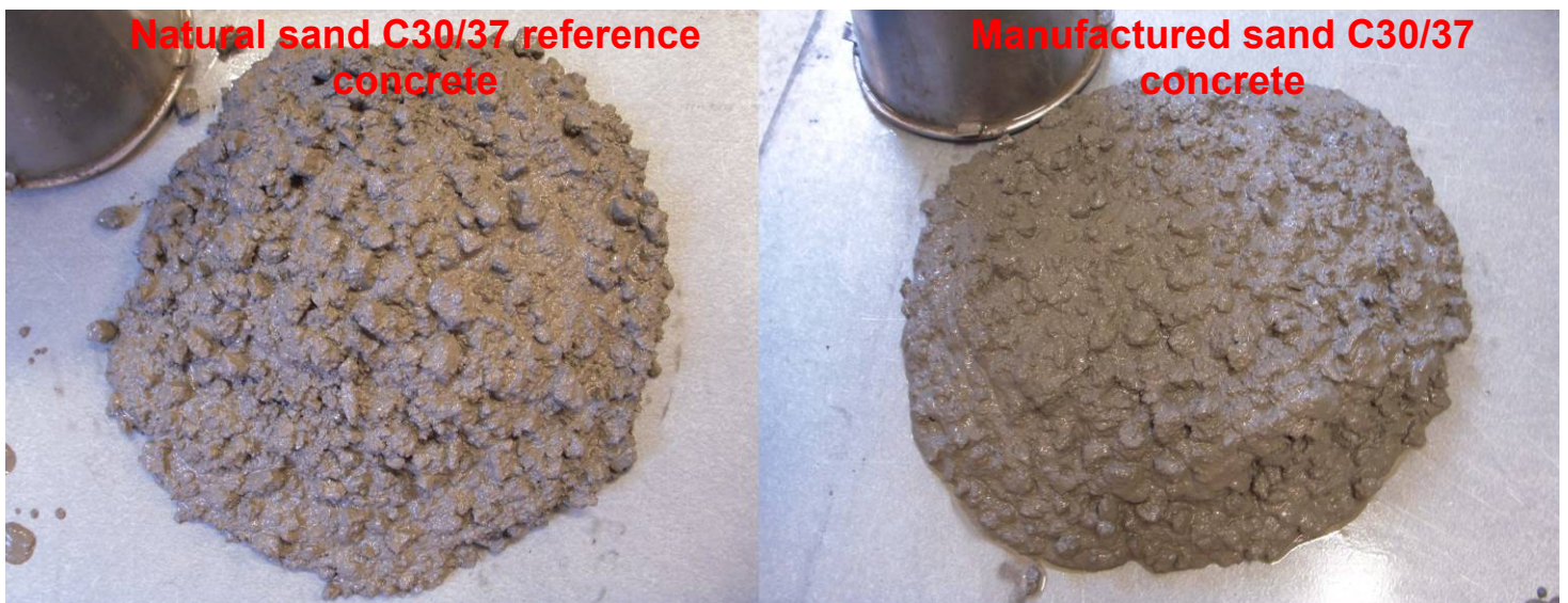
Figure 4-2 Slump-flow of the natural sand and manufactured sand C30/37 concrete
