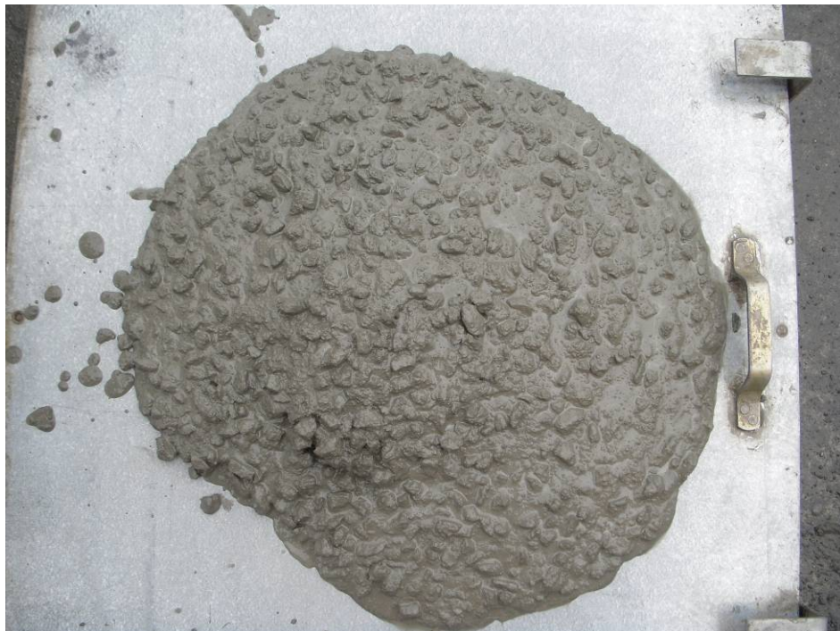
Figure 3-19 Grading R1-36 at a matrix volume of 394 l/m 3 (w/c=0.75)
