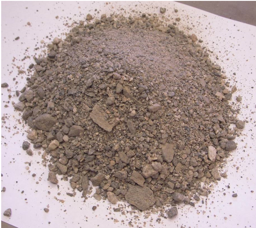
Figure 2-1 Naturally rounded glaciofluvial aggregate 0/8 mm used for concrete production in a mobile concrete plant in Jelsa quarry
