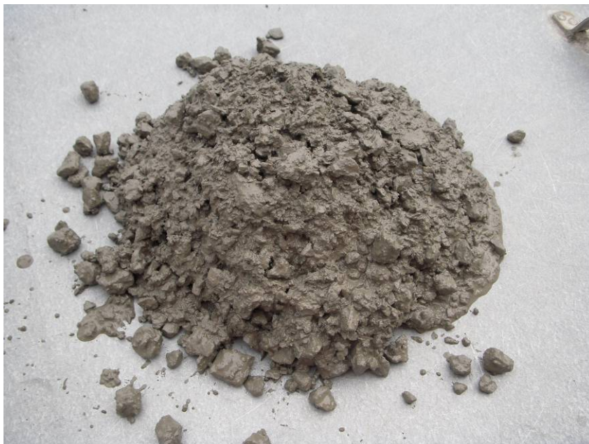
Figure 3-5 Grading R1-2 at a matrix volume of 350 l/m 3 (w/c=0.57)
