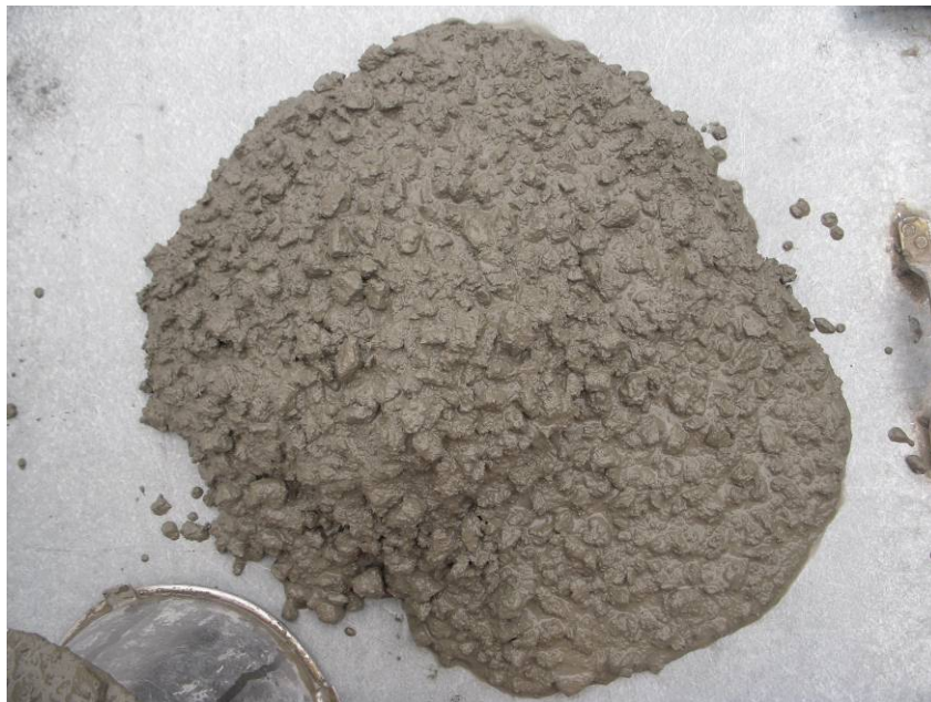
Figure 3-11 Grading R1-23 at a matrix volume of 394 \text{ l/m}^3 ( w/c=0.57 )
