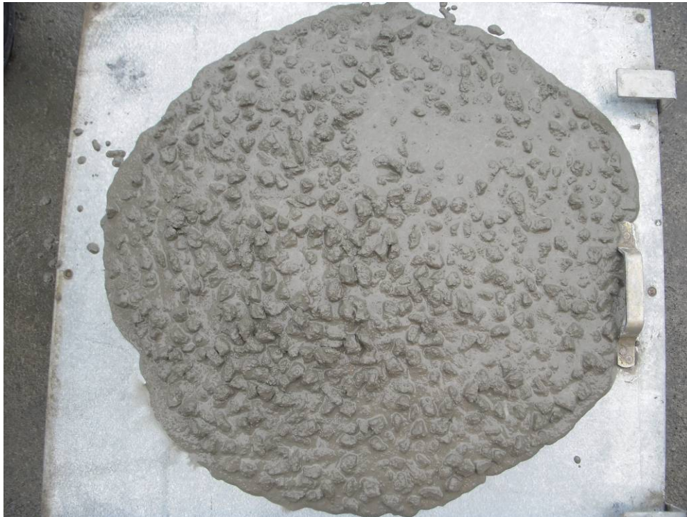
Figure 3-20 Grading R1-41 at a matrix volume of 427 l/m 3 (w/c=0.57) and slump-flow of 580 mm
