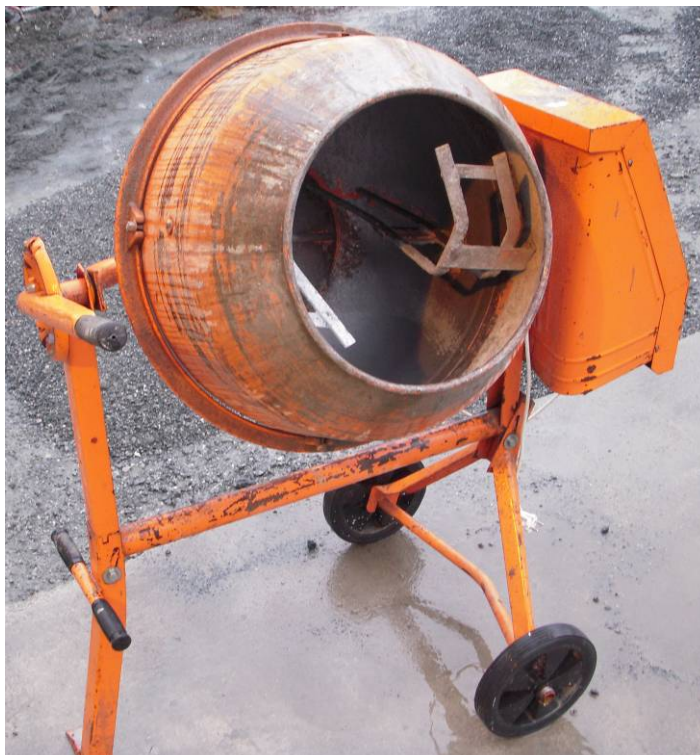
Figure 3-2 Free-fall mixer that was used to prepare the laboratory concrete mixes
