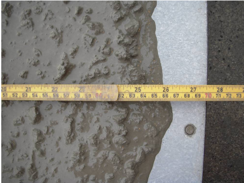
Figure 3-22 Grading R1-42 at a matrix volume of 444 \text{ l/m}^3 ( w/c=0.57 ) and slump-flow of 650 mm
