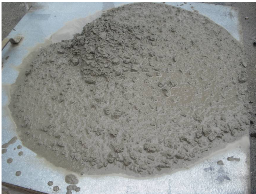
Figure 3-6 Grading R1-11 at a matrix volume of 410 l/m 3 (w/c=0.57)
