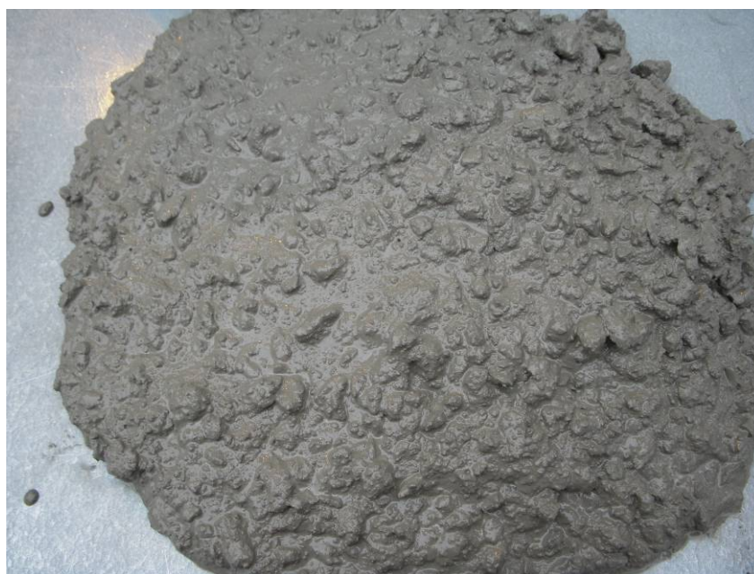
Figure 3-6 Grading R1-14 at a matrix volume of 442 l/m 3 (w/c=0.57)
