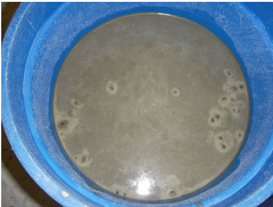
Figure 3-13 Bleeding test for mix R1-24; height of the concrete layer was 15 cm, picture taken about 2 hours after putting the concrete in the bucket
