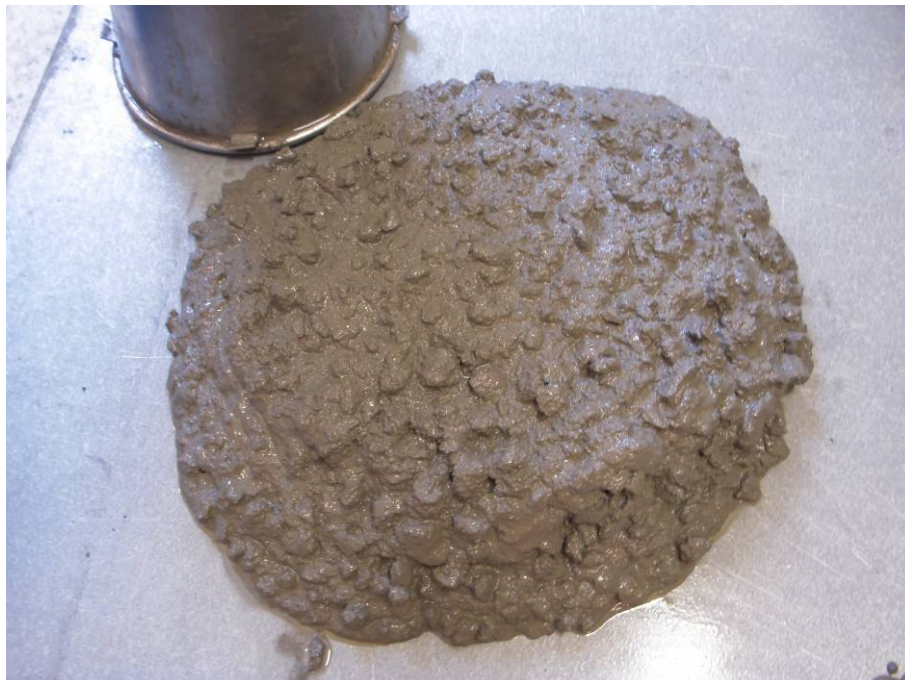
Figure 3-17 Grading R1-35 at a matrix volume of 400 \text{ l/m}^3 ( w/c=0.57 )
