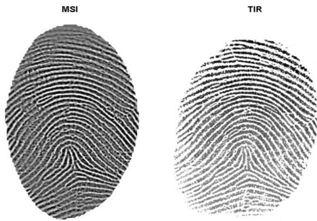
Figure 20 Example of TIR and composite multispectral image
