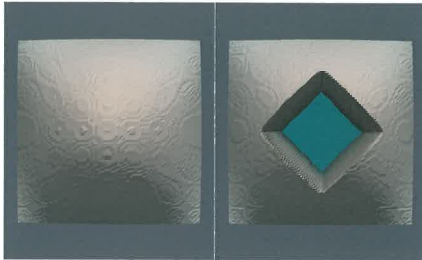
Figure 5: Excavation of a sinusoidal terrain with frequency 1 in both directions. Slopes of sidewalls are 45 degrees.
