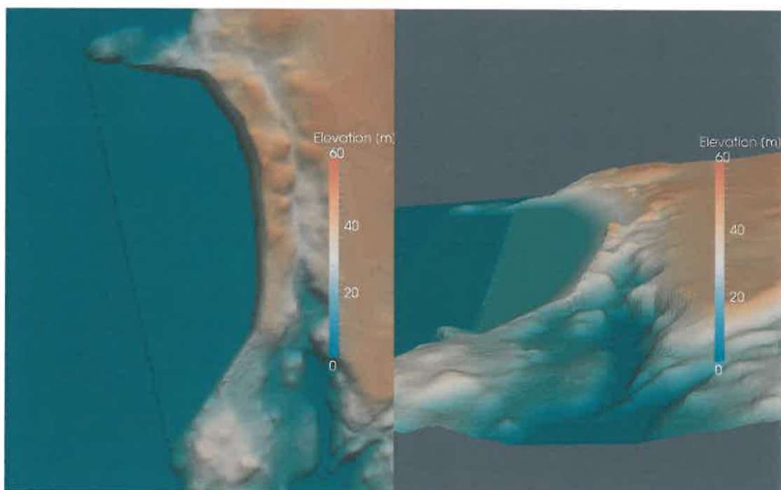
Figure 10: Excavated area by developed software based on the method described in Section 3. On the left is shown a harbour area at a single elevation, while the right side shows an example with two levels and an edge slope of 10^\circ at parts of the edge facing the runway.
