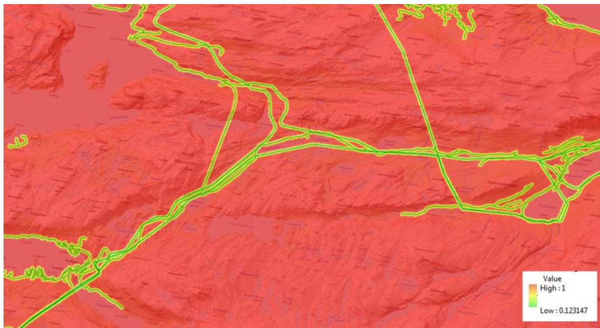
Figure 30. Example: Weight sum map for criteria 8a: Distance from roads, railways and power-lines (Bremanger municipality in western Norway).
