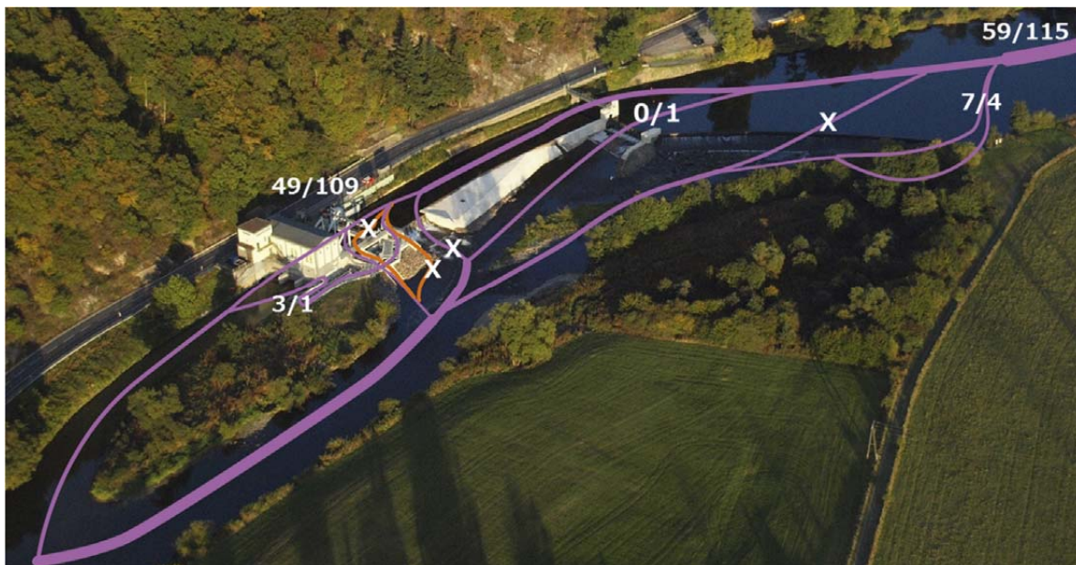
Figure 4.2. Numbers of smolt in 2014/2015 that used the different migration routes past the power station. Total number of smolt passing was 59 in 2014 and 115 in 2015. Water was not flowing over the dam or through the ice gate during the study, so these migration routes were not available (indicated with an X). Similarly, the bottom and side passes designed for eel were not in operation (orange lines, also indicated with an X). Water was flowing over the spillway gate only for short periods during the study in 2015, i.e. , 16 min - 5 hours on five occasions.
