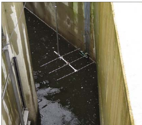
Figure 2.7. Detailed recording of the movements of tagged fish at the power stations was done by using a network of stationary receivers with antennas covering all possible migration routes. Lotek model SRX 600 data loggers were used with 3-, 4-, 6- and 9-element Yagi-antennas or co-axial antennas used underwater or in air. When a tagged fish was within the detection range of an antenna, date, time, individual fish code, signal strength from the transmitter and individual antenna number were automatically recorded and stored by the receiver and later downloaded to a computer. Photos from Unkelmühle, by Eva B. Thorstad and Stein Are Sæther.
