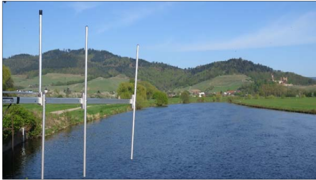
Figure 2.6. Downstream migration of tagged fish was studied by using stationary receivers, which automatically stored information on time and id of tagged fish when they were within the detection range of receiver antennas. Photos from the Kinzig (left) and the Sieg (right) by Eva B. Thorstad.
