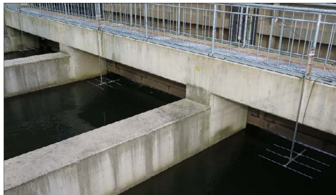
Figure 2.7. Detailed recording of the movements of tagged fish at the power stations was done by using a network of stationary receivers with antennas covering all possible migration routes. Lotek model SRX 600 data loggers were used with 3-, 4-, 6- and 9-element Yagi-antennas or co-axial antennas used underwater or in air. When a tagged fish was within the detection range of an antenna, date, time, individual fish code, signal strength from the transmitter and individual antenna number were automatically recorded and stored by the receiver and later downloaded to a computer. Photos from Unkelmühle, by Eva B. Thorstad and Stein Are Sæther.
