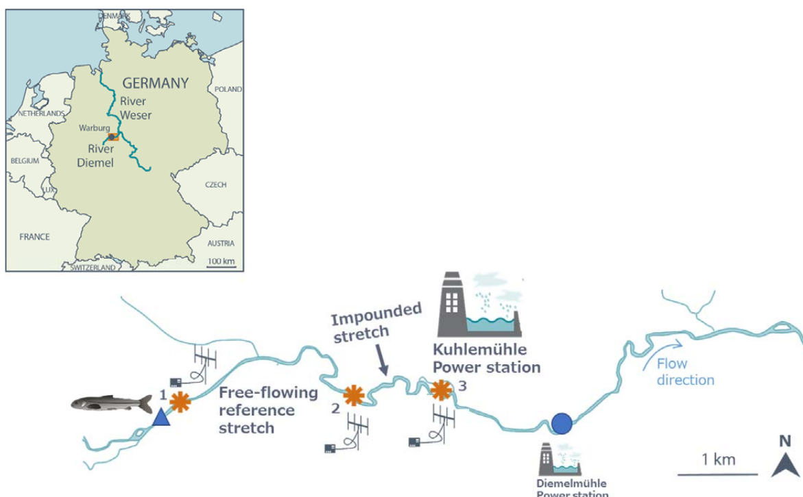
Figure 3.10. Study area in the Diemel showing the release site of Atlantic salmon smolt tagged with radio transmitters (blue triangle), receiver sites where they were recorded when passing (orange stars, denoted with site numbers 1-4) and the Kuhlemühle power station. Diemelmühle power station is also shown on the map, but no receivers were installed to monitor smolt at this site.
