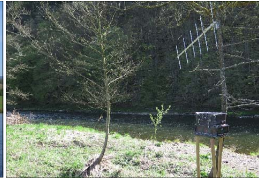
Figure 2.6. Downstream migration of tagged fish was studied by using stationary receivers, which automatically stored information on time and id of tagged fish when they were within the detection range of receiver antennas. Photos from the Kinzig (left) and the Sieg (right) by Eva B. Thorstad.
