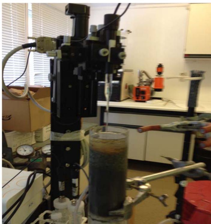
Figure 3. Set up for microsensor depth profile measurements of O_2 , H_2S and pH, showing O_2
