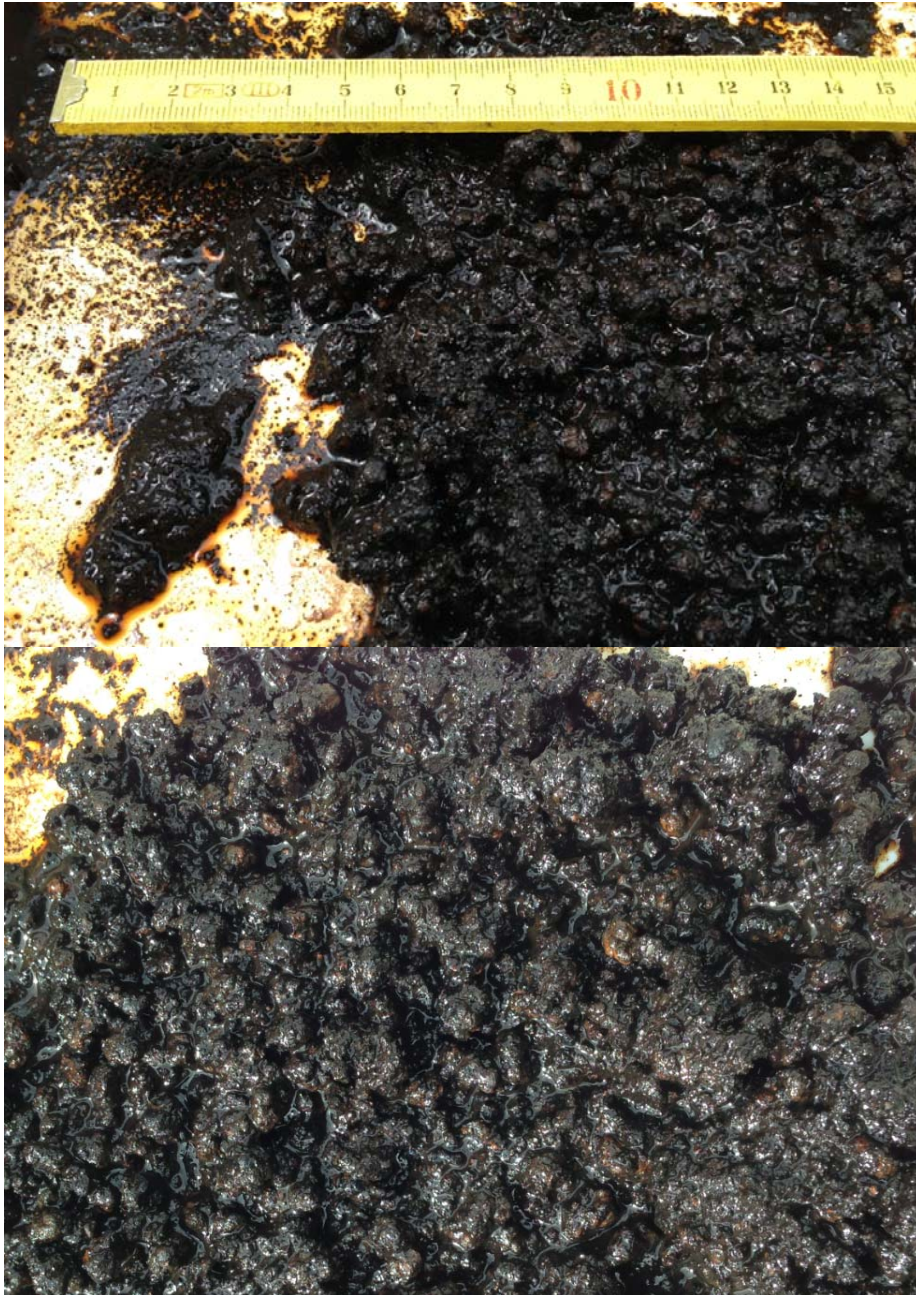
Figure 9. Fresh sediment collected with the grab sampler for invertebrates at Lake Breisjøen. Loose organic material was removed by gentle flushing, in order to visualize that the vast majority of the sample was metal nodules. The black colour is caused by Mn oxides and the brown-orange of oxidized Fe.
