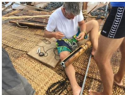
Figure 20 Nortek Aquadopp instrument mounted on Rahiti Tane to measure seawater current strength and direction. It was installed inside a bamboo for protection.
