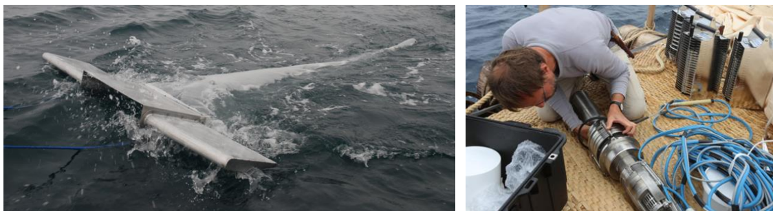
Figure 27 The Manta Trawl (left) and the three-stage sampler were installed on Tupac Yupanqui to collect micro plastic samples throughout the cruise. In the right, Håkon assembles the filtering water pump for the sampler.
