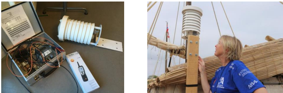
Figure 17 Weather station components are shown on the left. The equipment was provided by Aslaug Mariolijn van Nes from the Norwegian Meteorological Institute. The weather station installed on Rahiti Tane was used to report meteorological information every six hours.
