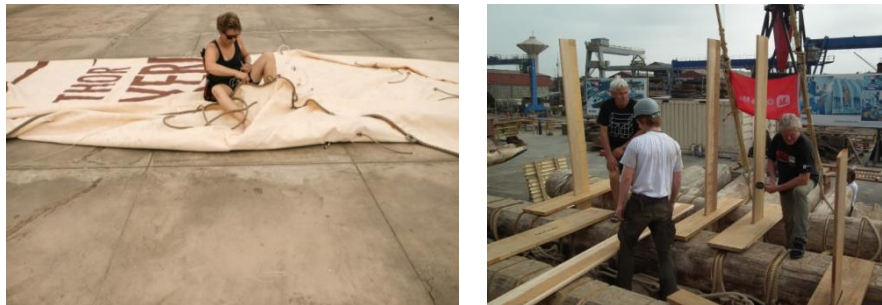
Figure 3 On the left, Gunvor reinforces the sail of Tupac Yupanqui. Builders on the right test the guara setup on the deck of a raft.
