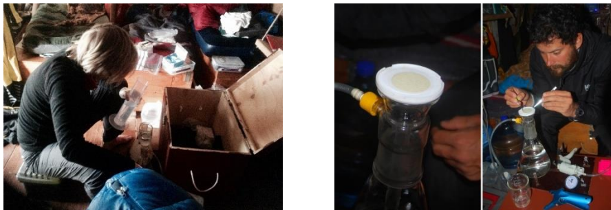
Figure 24 On the left, Cecilie filters Chlorophyll A and DNA from sea water on the first leg of the expedition. Pedro De La Torre on the right continued this procedure and a sample with Chlorophyll A is shown in the middle.
