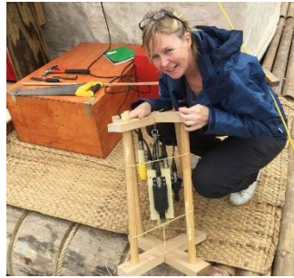
Figure 18 Cecilie demonstrates the wooden frame built to protect the surface CTD that was permanently deployed under the Rahiti Tane raft.
