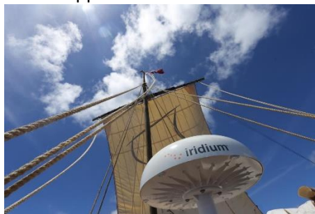
Figure 9 The Iridium Pilot antenna was installed on Tupac Yupanqui for faster satellite internet access
