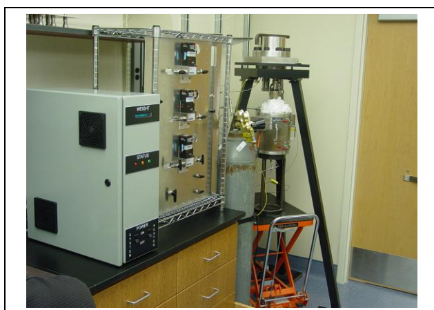
Figure 3-3. RTI high-pressure TGA (HP TGA) modified for testing CO 2 sorbent materials
