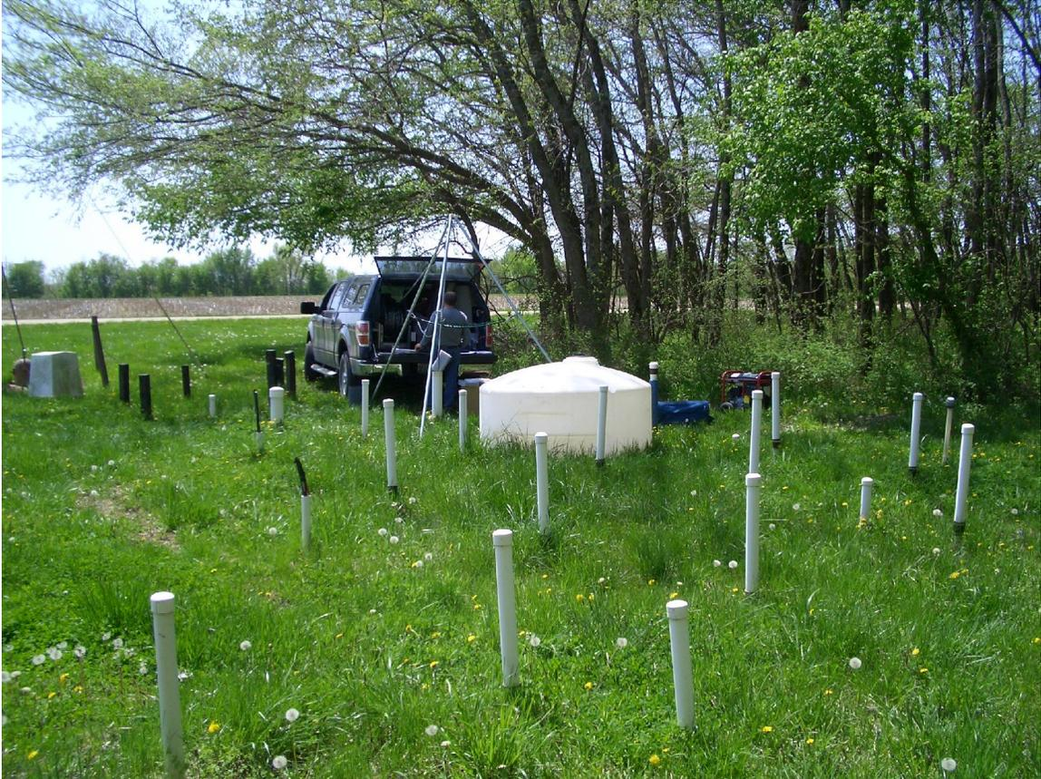
**Figure 17: Vista Clara employee Igor Frid monitoring an NMR logging experiment in GEMS well #4S, April 19 2010.**
