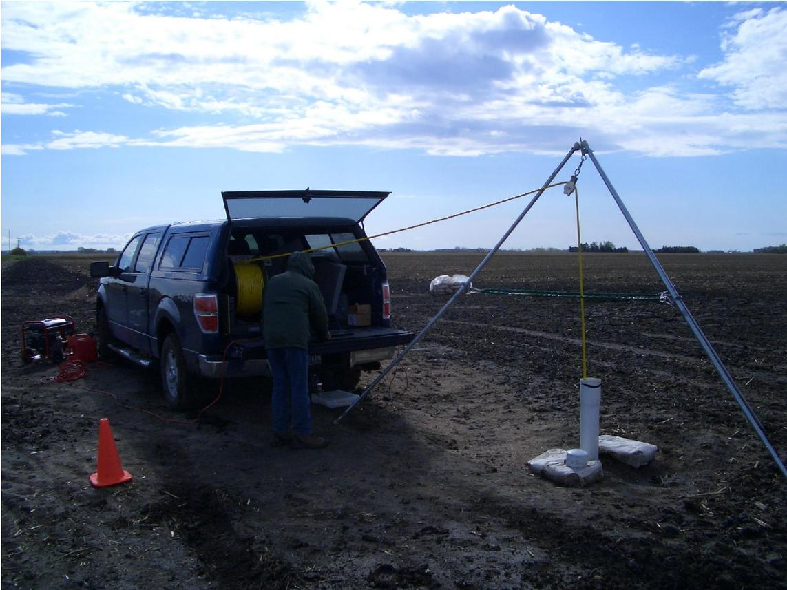
**Figure 8: Borehole NMR instrument at site 58b. Lexington NE, April 24, 2010.**
