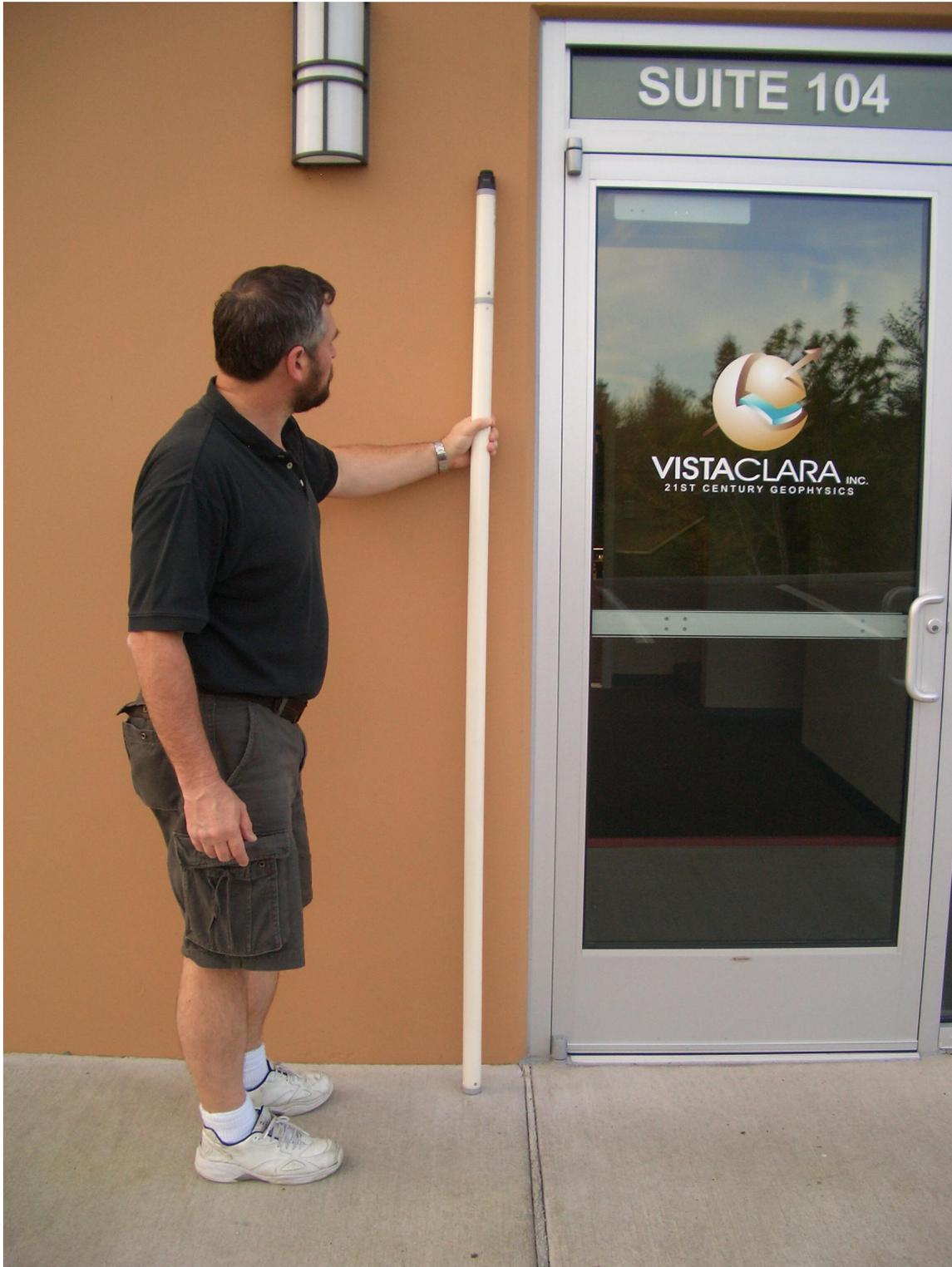
Figure 32: Photo of 1.67” diameter borehole NMR probe.
