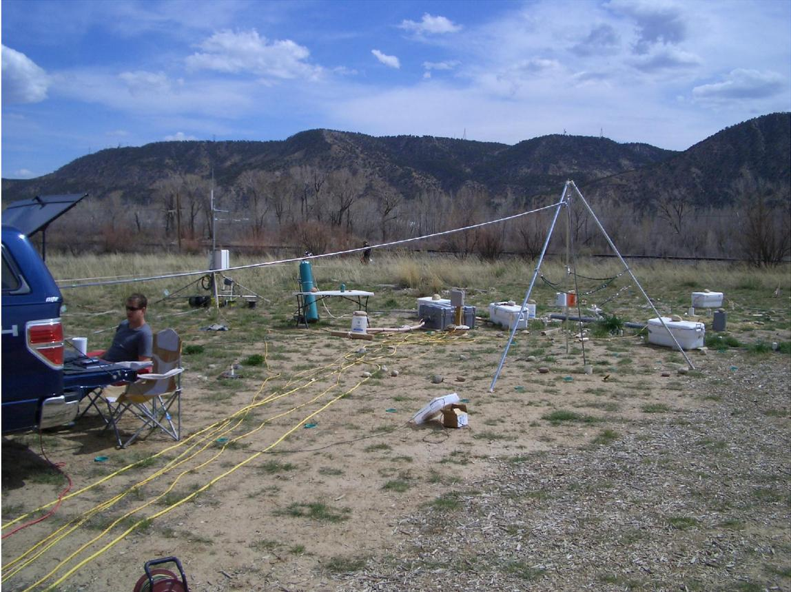
**Figure 11: NMR logging of borehole #U02, on April 16, 2010. Note the proximity of other measurement instrumentation and power lines.**
