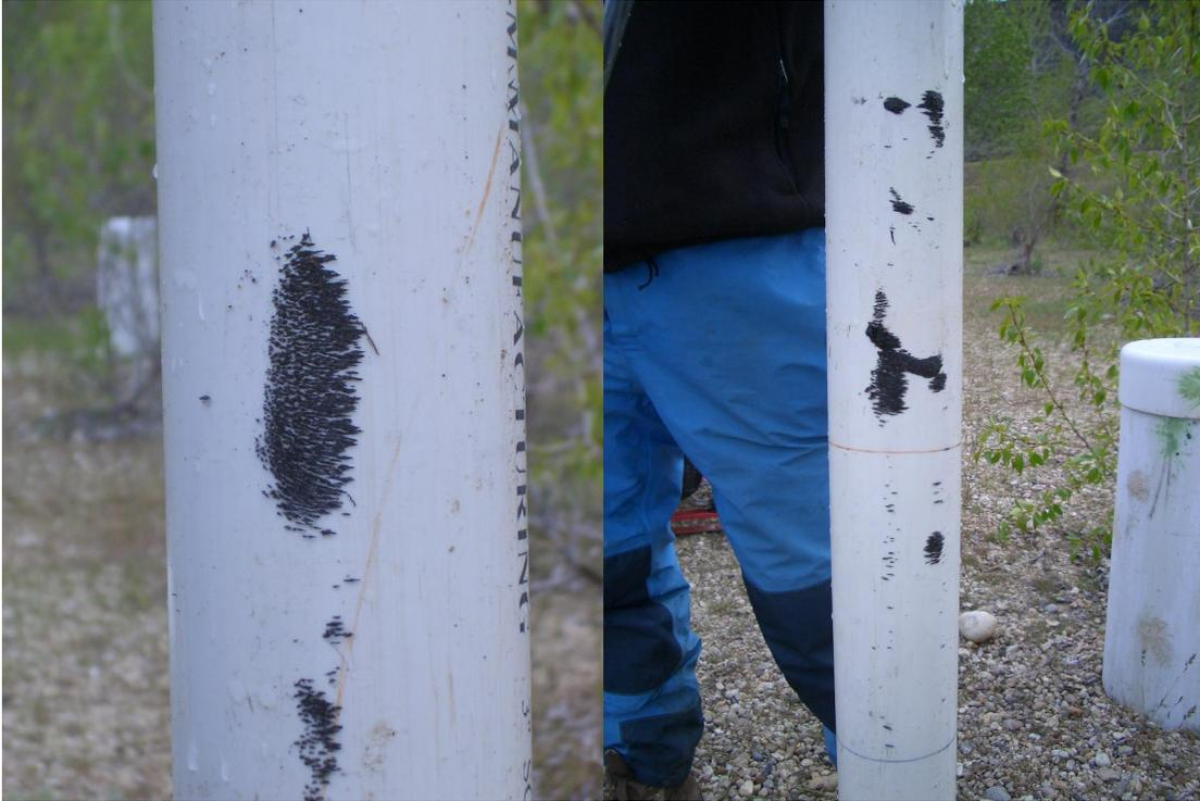
**Figure 24: Iron-rich particles clinging to the NMR probe after raising it from the well in Boise ID.**
