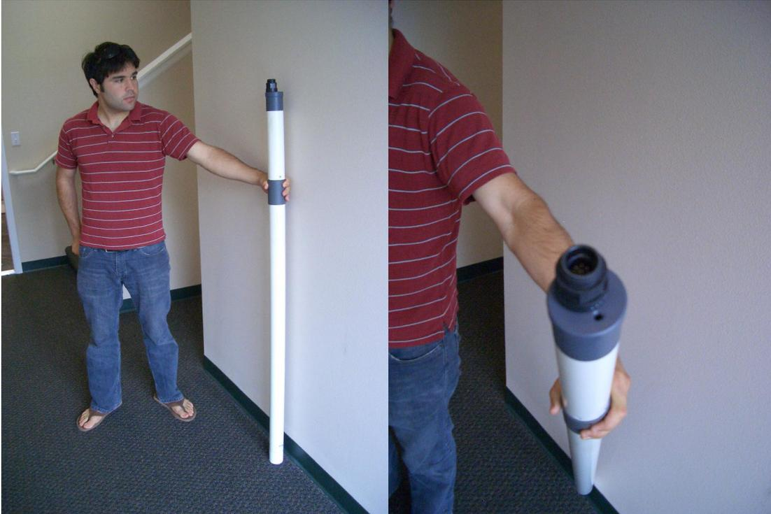
**Figure 35: Geoprobe-supplied packaging for direct push NMR logging. Photo at right shows the waterproof cable connector we are using on all NMR probes.**
