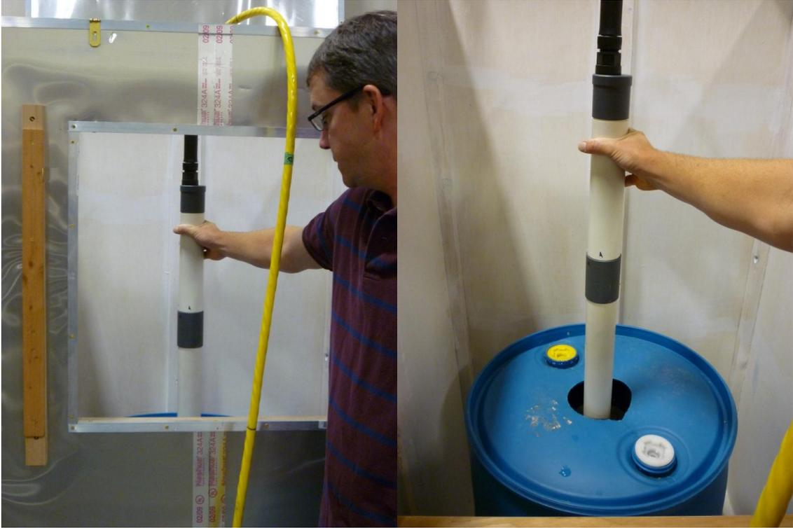
**Figure 33: Calibration tank used for testing and calibrating the response of individual probes to water content of 50% or 100%. The 2.5" Geoprobe probe is shown in this photo. The blue 55 gallon plastic barrel is filled with water.**
