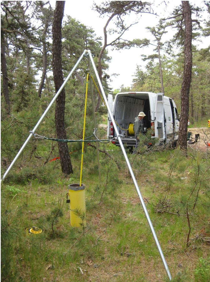
**Figure 29 NMR instrumentation at MMR well #FSW 545-0060.**
