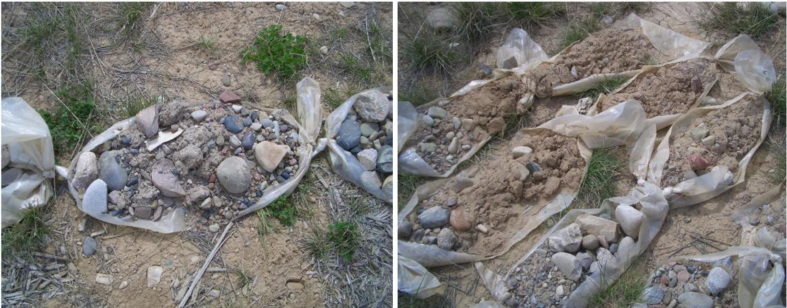
**Figure 12: Drilling samples arranged on the ground in the vicinity of borehole U02.**
