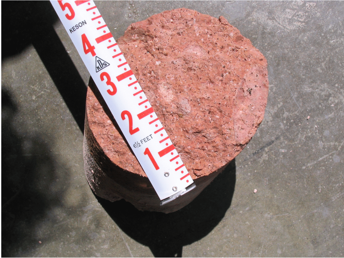
Figure 4-16 Close-up Photographs of Core of Redrock Valley Tuff from Hydrologic Test Hole U-3cn#5
