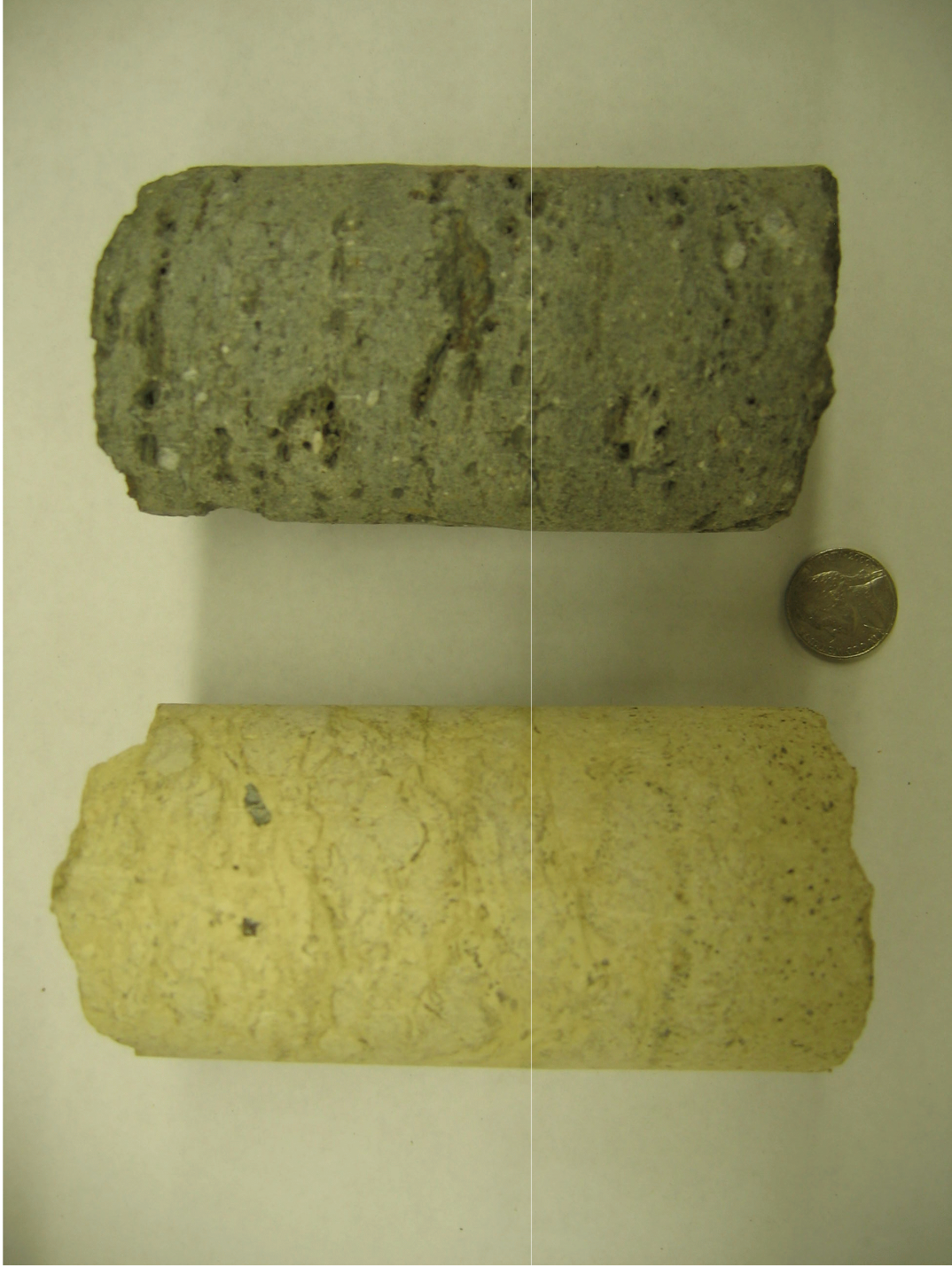
Figure 4-5 Comparison of Welded Grouse Canyon Ash-Flow Tuff (Tbg) from Exploratory Hole UE-12t#3 (right) and Zeolitic, Bedded Grouse Canyon Ash-Fall Tuff (Tbgb) from Exploratory Hole UE-7f (left)
