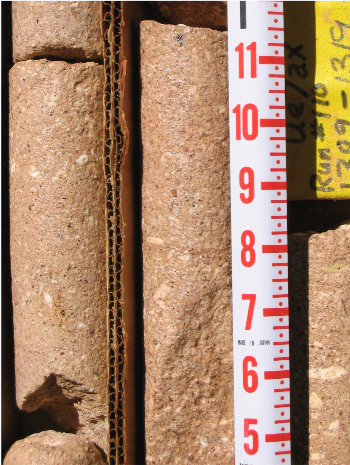
Figure 4-18 Close-up Photograph of Core of Tuff of Twin Peaks from Exploratory Hole UE-7ax
