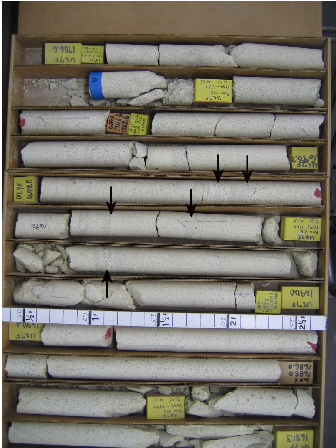
Figure 4-4 Zeolitic Bedded Grouse Canyon Tuff (Tbgb) in Core from Exploratory Hole UE-7f (Black arrows indicate bedding planes)
