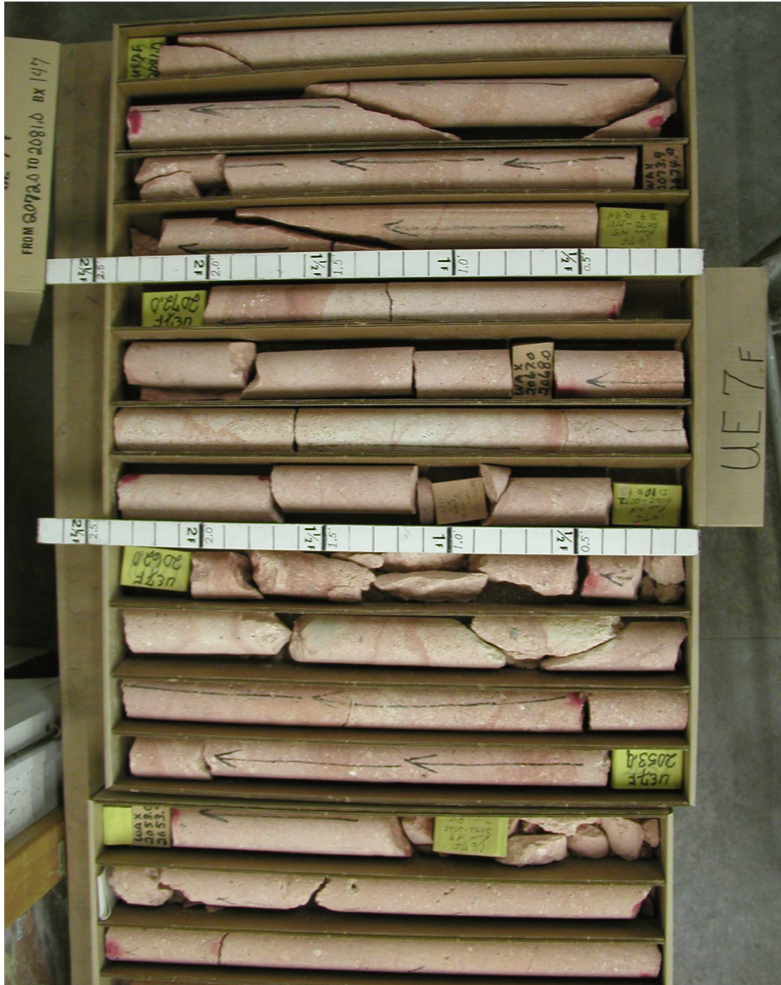
Figure 4-8a Zeolitic, Nonwelded Tunnel Bed 3BC-Equivalent from Exploratory Hole UE-7f (Depth 2,050–2,081 ft)
