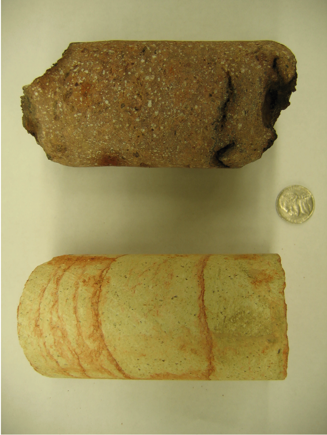
Figure 4-12 Comparison of Welded Tub Spring Ash-Flow Tuff from Exploratory Hole UE-12t#3 (right) and Zeolitic Tub Spring Ash-Fall Tuff from Exploratory Hole UE-7f (left)
