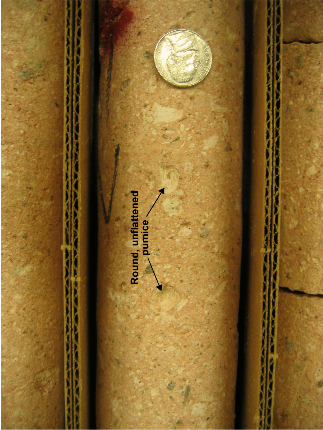
Figure 4-7 Close-up Photograph of Core of Tn4E-Equivalent Nonwelded Ash-Flow Tuff from Exploratory Hole UE-7f
