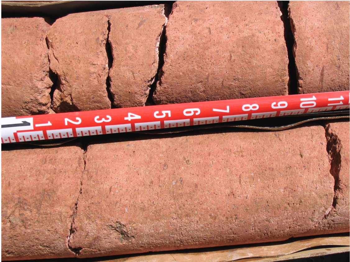
Figure 4-16 Close-up Photographs of Core of Redrock Valley Tuff from Hydrologic Test Hole U-3cn#5
