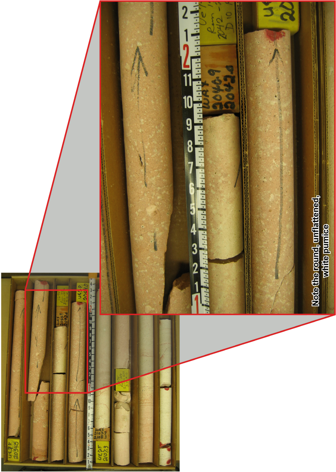
Figure 4-8b Zeolitic, Nonwelded Tunnel Bed 3BC-Equivalent from Exploratory Hole UE-7f (Depth 2,034-2,116 ft)
