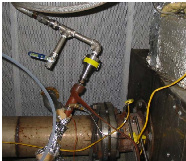
Figure 3-12. Photo of sampling apparatus (Credit: NREL ReFUEL Laboratory photos)
