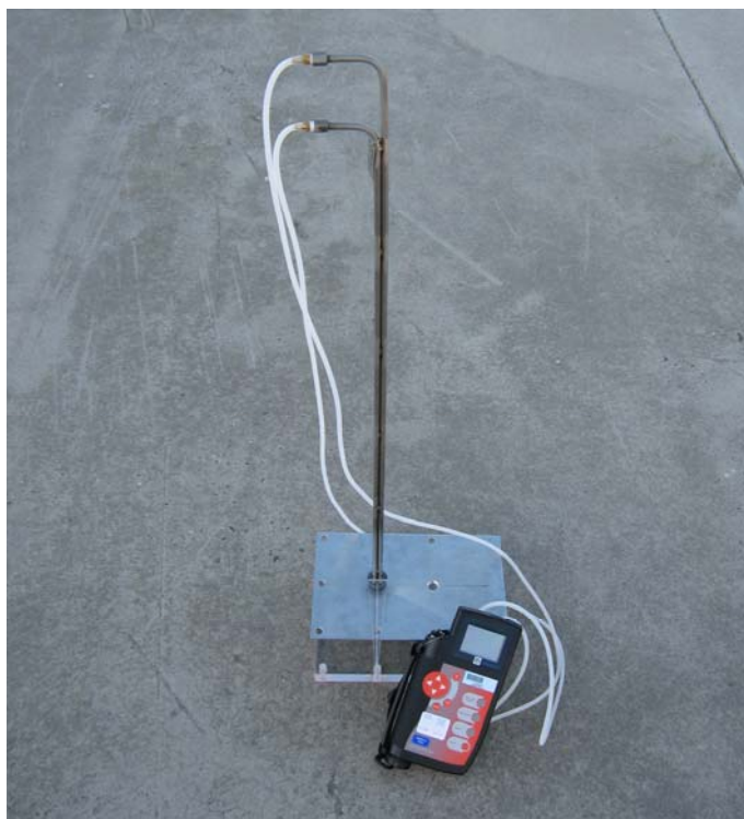
Figure 3.5. Electronic Manometer Connected to Pitot Tube
