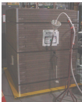
The underground shield for the low energy threshold germanium detector and a cut away schematic view.
