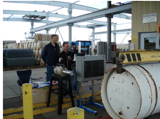
Measurement with NaI He-3 detector suite representative of integrated cylinder verification station instrumentation.
