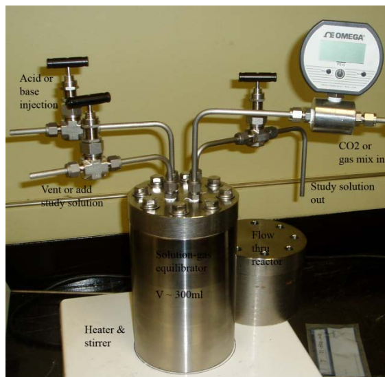
Figure 5. Photograph of titanium brine- \text{CO}_2 reactor.
