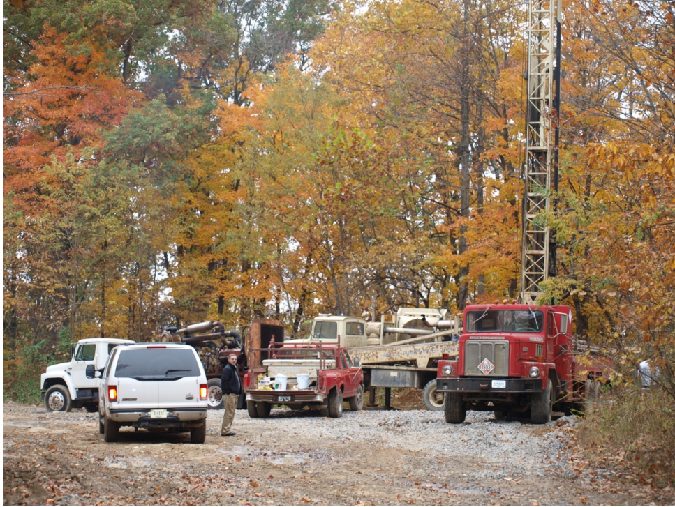
Figure 9. Drilling operation at Ft. Knox showing the size of the area required for establishment and conducting drilling operations.
