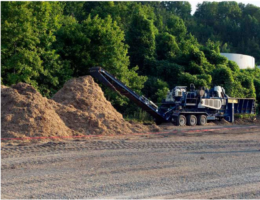
Figs. 5.2 and 5.3. Approximately 1500 yd 3 of mulch was created from trees and brush that were cleared during construction of a new bypass road. This mulch was then put inside fabric bags for use as erosion control devices. This project illustrates the reuse of natural resources in order to protect other natural resources.
