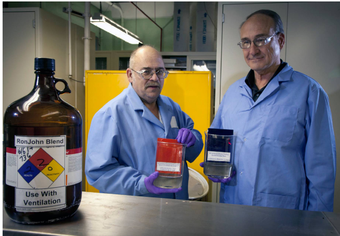
Fig. 5.1. Y-12 research chemist Ron Simandl and laboratory assistant John Brown developed a non-hazardous solvent blend (RonJohn Blend) that can effectively soften polyurethane adhesives, enabling workers to separate parts more quickly and with less effort.
