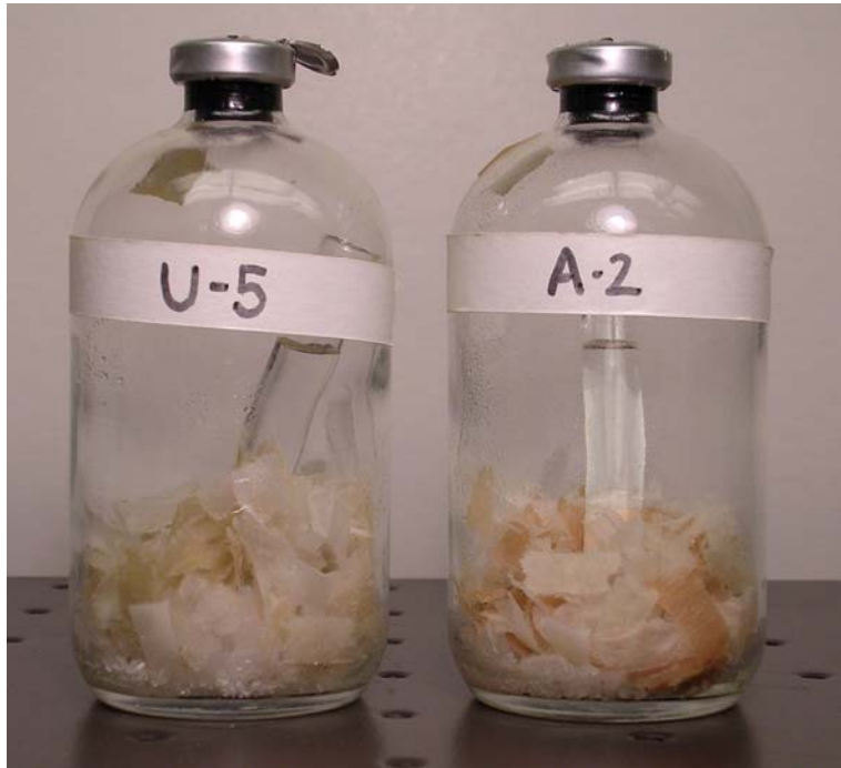
Figure 16(a). Initially aerobic humid samples at 3334 days (9.1 years) incubation: unamended inoculated (U-5) and amended inoculated (A-2). Some discoloration of the paper is evident in U-5.
