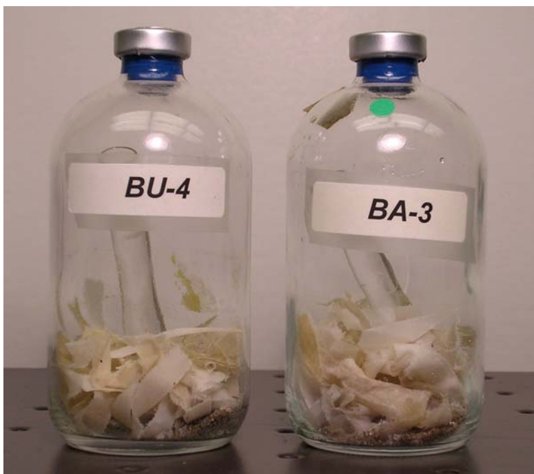
Figure 19 (b). Anaerobic humid samples with bentonite at 2945 days (8.1 years) incubation: unamended inoculated (BU-4) and amended inoculated (BA-3). Discoloration of the paper is evident in both treatments, as well as a red biofilm in the bentonite at the bottom of the bottles.
