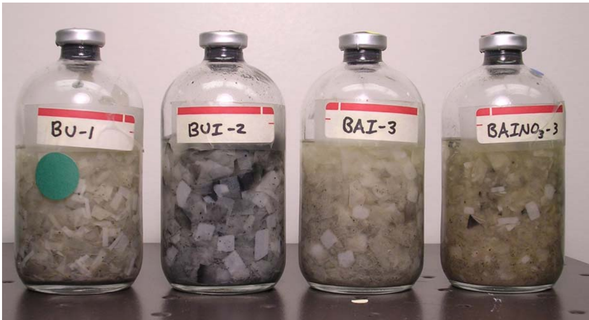
Figure 8(b). Photograph of anaerobic samples with bentonite at 3929 days (10.8 years) incubation: unamended uninoculated (BU-1), unamended inoculated (BUI-2), amended inoculated (BAI-3), and amended inoculated plus excess nitrate (BAINO 3 -3). Blackening in BUI-2 and BAINO 3 -3 is due to iron sulfide. Discoloration of brown paper is evident in BU-1.
