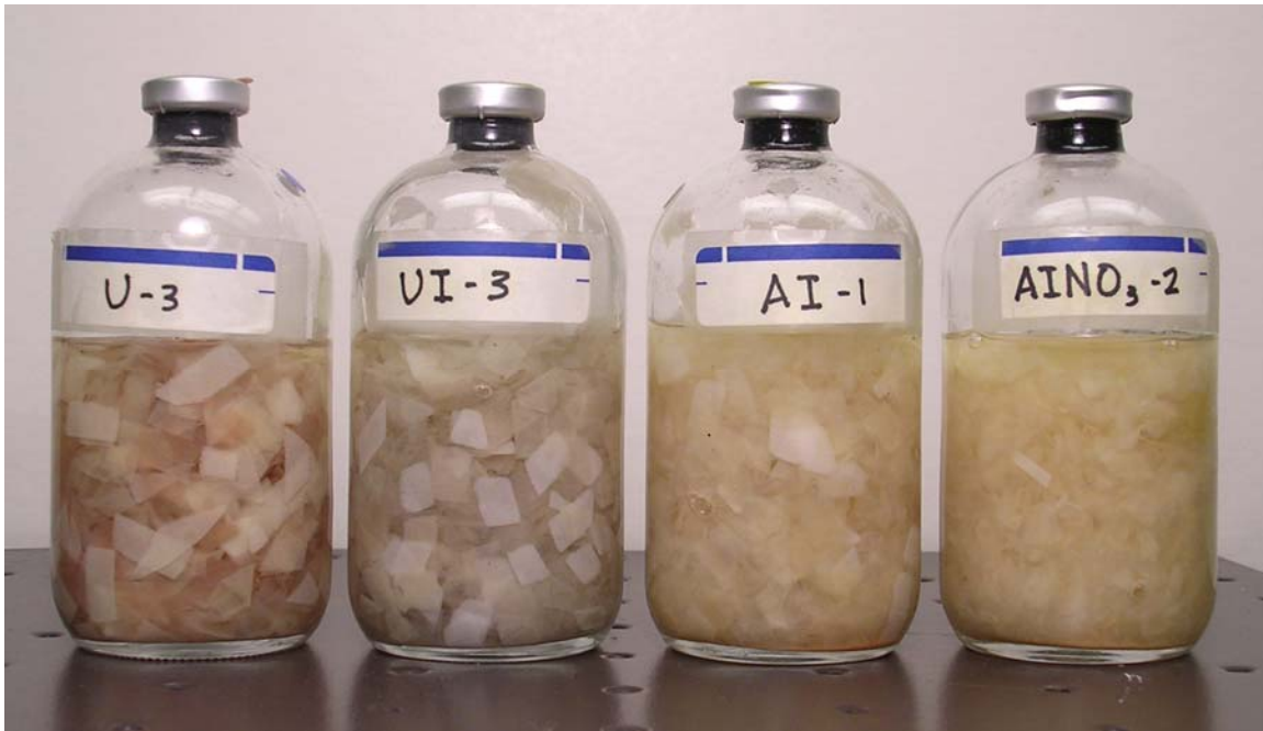
Figure 5(a). Photograph of aerobic samples at 3929 days (10.8 years) incubation: unamended uninoculated (U-3) , unamended inoculated (UI-3), amended inoculated (AI-1), and amended inoculated plus excess nitrate (AINO 3 -2). Degradation of the cellulose is evident in AI-1 and AINO 3 -2 samples as shown by pulping of the squares of paper.
