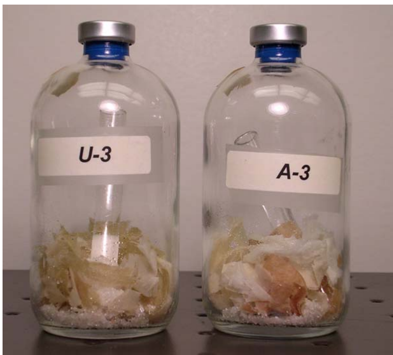
Figure 19 (a). Anaerobic humid samples at 2945 days (8.1 years) incubation: unamended inoculated (U-3) and amended inoculated (A-3). The brown paper in U-3 has become discolored.
