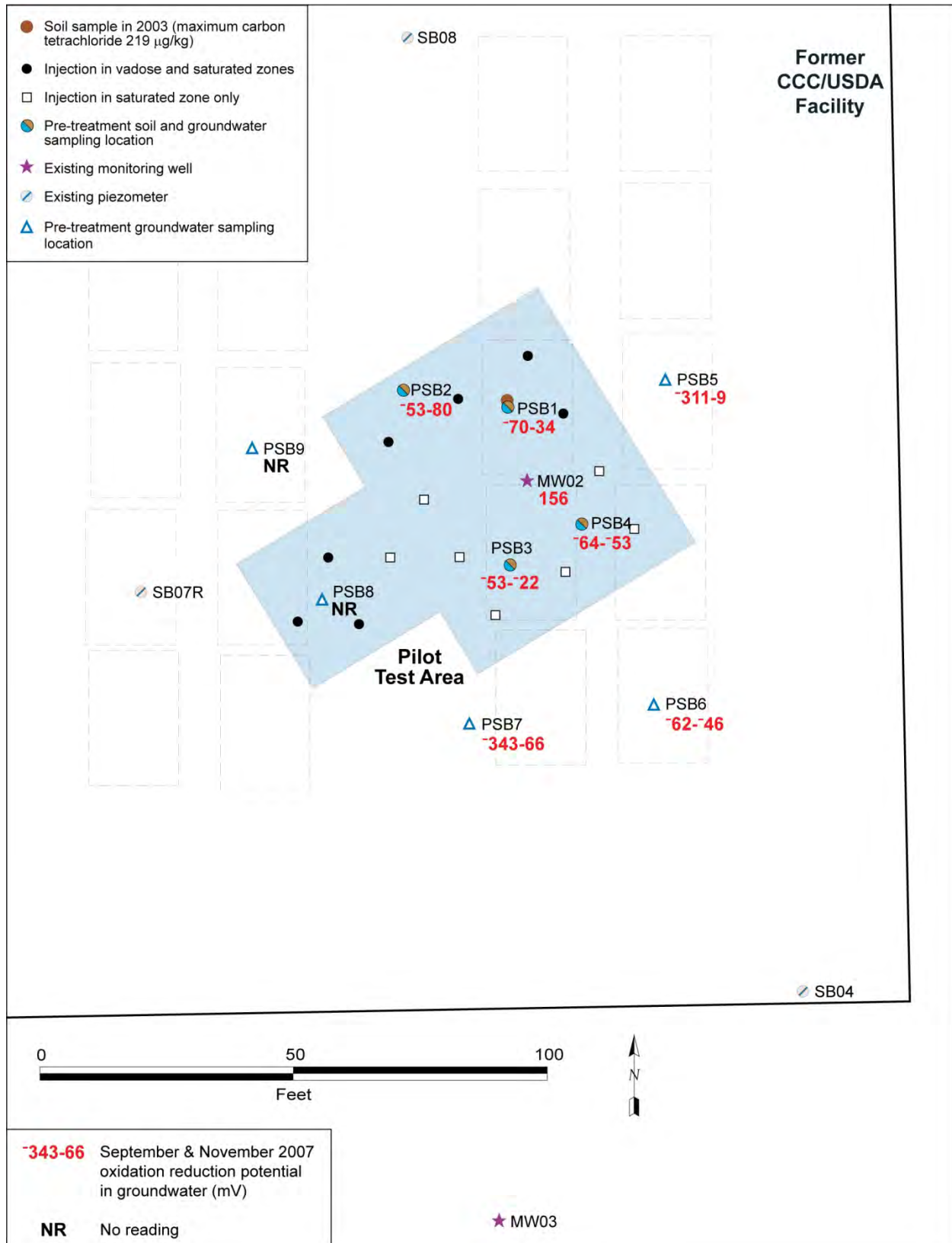
FIGURE 3.6 Field-measured results for ORP in groundwater samples collected during the pre-injection baseline sampling, September and November 2007.
