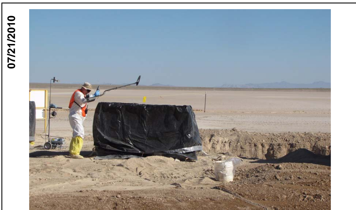
Figure 3-3 UXO Technician Using Analog Magnetometer To Check for UXO in Waste Container
