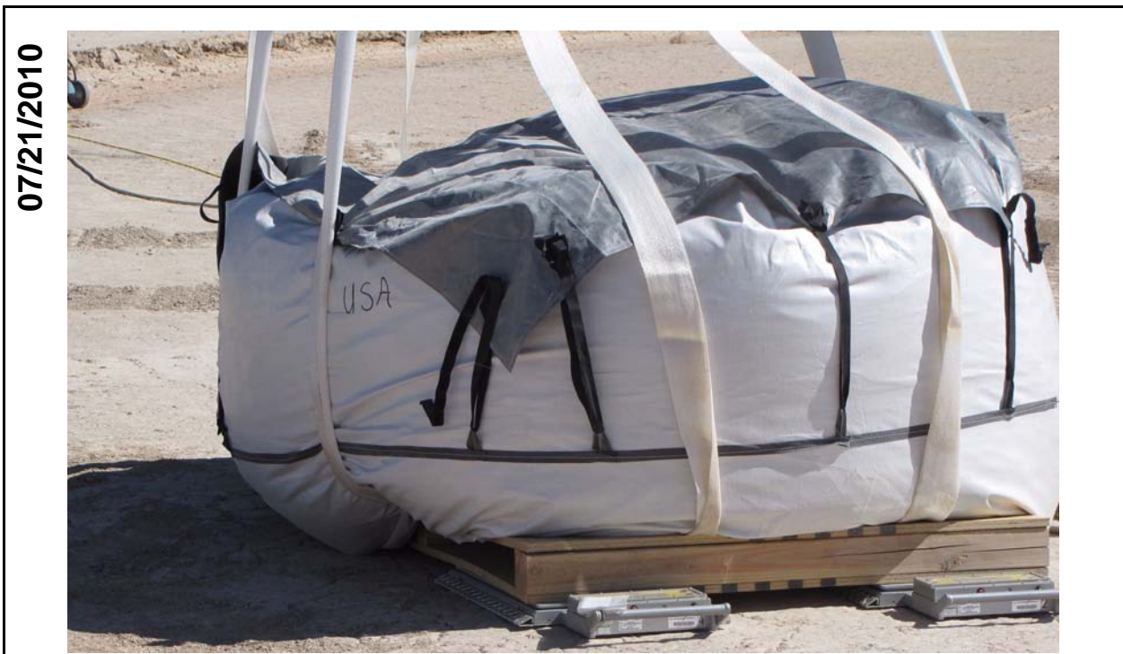
Figure 6-2 5-yd 3 Super Sack Being Weighed before Shipment for Disposal
