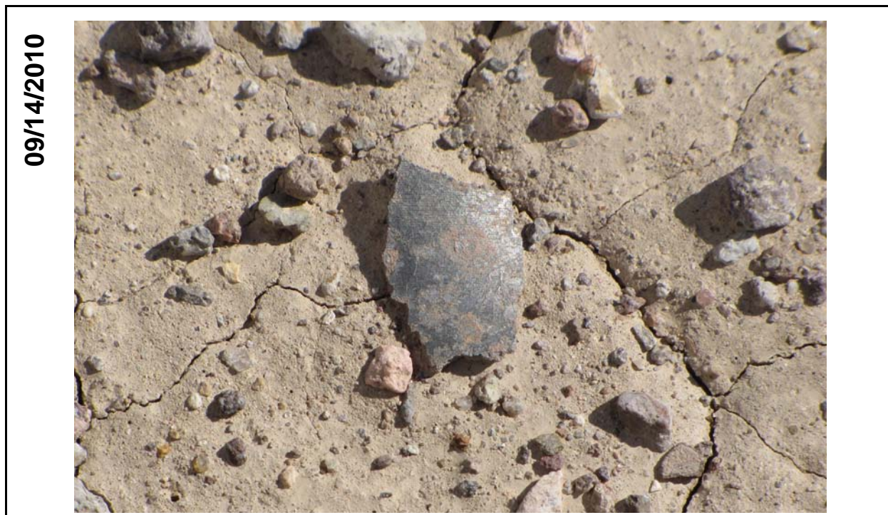
Figure 5-2 Close-up View of DU Fragment on Soil Surface at NEDS Lake
