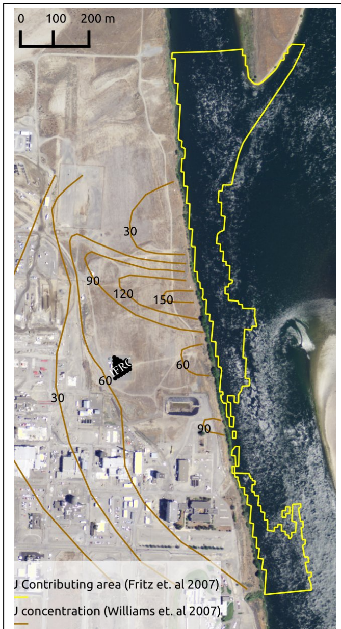
Figure 4. U concentration in the 300 Area, and estimated U contributing area [Fritz et al., 2007]
