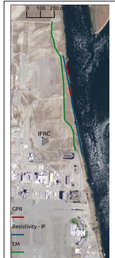
Figure 17. Location of the trial GPR, EM and Resistivity – IP land borne surveys
