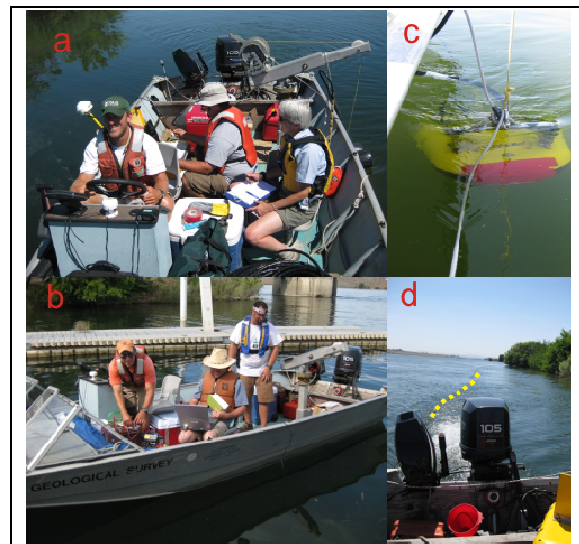
Figure 11. Water-borne geophysical data collection: a) GPR – seismic, and b) \rho / IP field crews; c) chirp seismic unit, d) \rho / IP survey showing towable graphite electrode string (yellow dots superimposed on electrodes for clarity).
