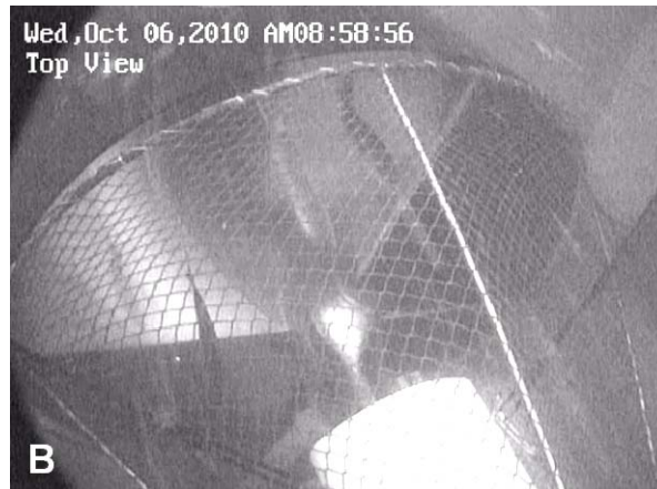
Figure 3-6 Side camera view (A) showing a fish being struck by a blade and top view (B) showing fish swimming immediately upstream of the blade sweep during testing at an approach velocity of 1.5 m/s.
