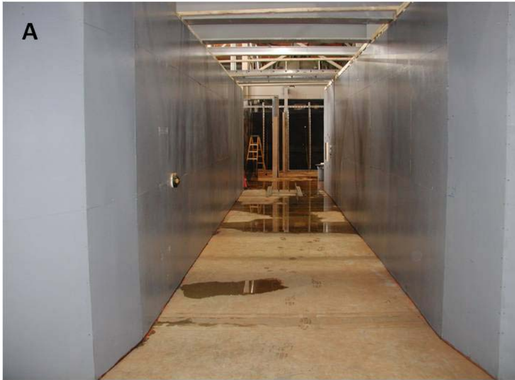
Figure 2-6 Downstream View (A) and Upstream View (B) of Alden's large flume fish testing facility configured for the biological evaluation of hydrokinetic turbines with constricting walls installed
