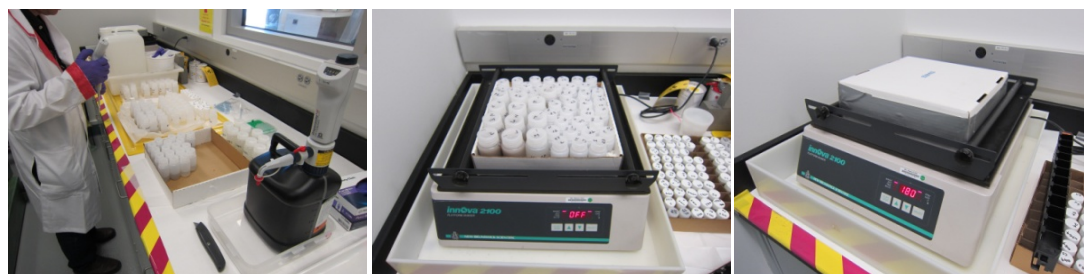
Figure 6 Placement of test samples in a container box and on the shaker table
