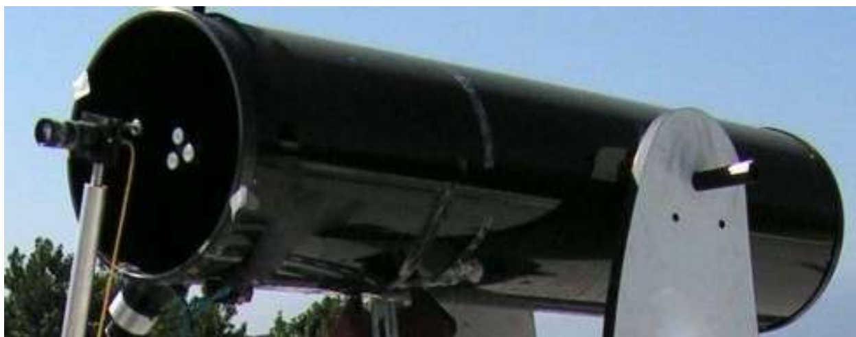
Figure 7. 8" Large aperture transceiver based on a commercial telescope.
