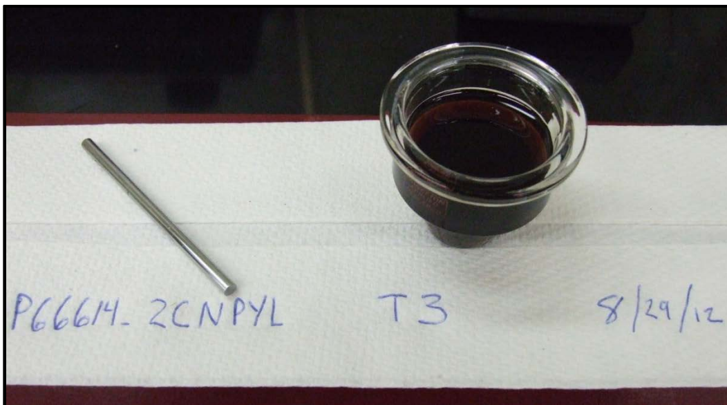
Figure 8.10: Post-Test 3 IL NDIL0046, CO 2 , and 1018-CS Test Specimen
