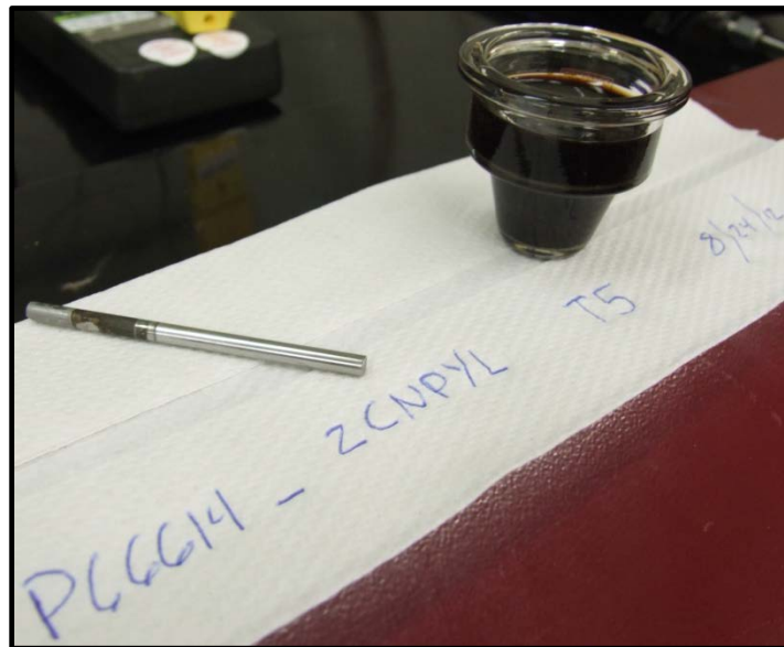
Figure 8.14: Post-Test 5 Neat IL NDIL0046 and 1018-CS Test Specimen
