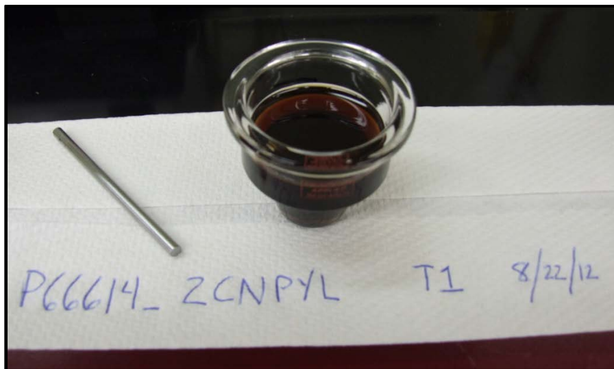
Figure 8.6: Post-Test 1 Neat IL NDIL0046 and 1018-CS Test Specimen
