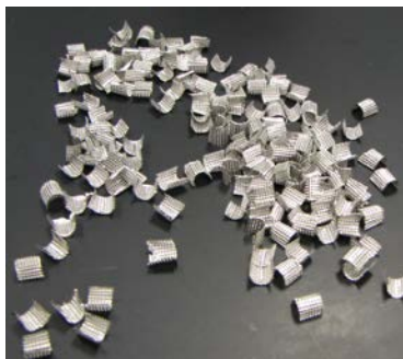
Figure 5. Laboratory Random Packing
