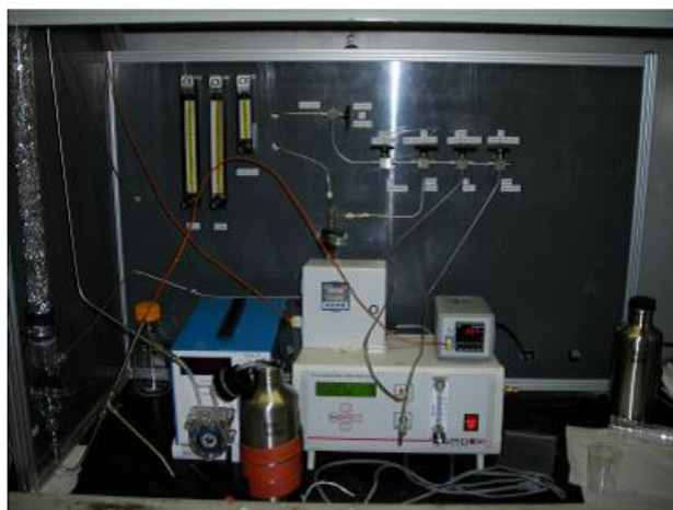
Figure 60: Photo of bench-scale test system. The glass packed column is on the left, CO 2 detector in foreground and associated piping and valves in the background.
