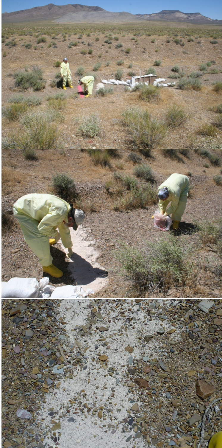
Figure 9. At installation, the pebbles (pea gravel) and sand placed in the channel above the flume at the Smoky Site thoroughly covered the channel bed and had a nearly straight downstream edge (top two images). The lower photo, taken July 2012, shows irregularity in the downstream edge of the sand and native gravel on top of the sand.
