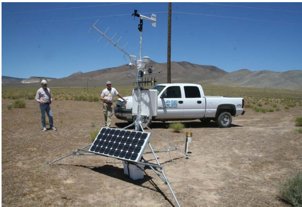
Figure 3. Smoky CA meteorological station was installed to measure precipitation, wind and other climate parameters.
