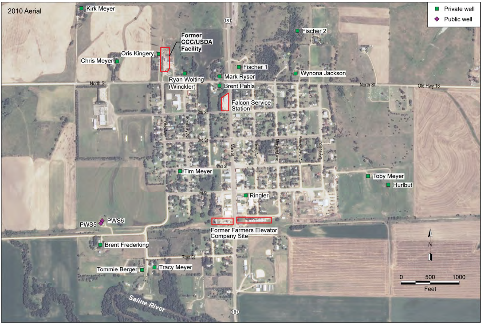
FIGURE 2.1 Locations of the former CCC/USDA facility, the Falcon Service station (previously owned by Feldkamp Brothers Oil Company), the former Farmers Elevator Company site, and adjacent private wells and public water supply wells. Locations of private wells are estimated on the basis of the KDHE (1998) investigation report, Kansas water well registration forms, and communications with Sylvan Grove officials. Sources of photograph: NAIP (2010).
