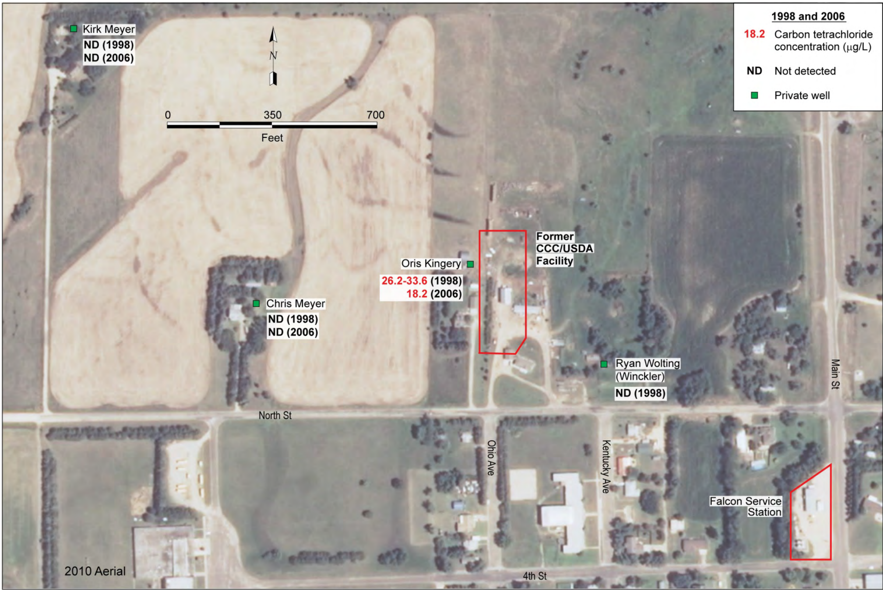
FIGURE 2.2 Historical analytical results for carbon tetrachloride in groundwater samples collected by the KDHE in 1998-2006 from four private wells near the former CCC/USDA facility. Source of photograph: NAIP (2010).
