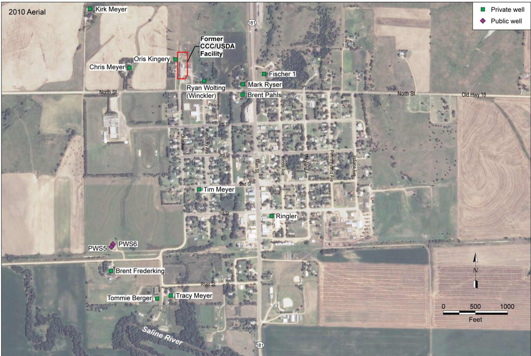
FIGURE 3.2 Proposed groundwater sampling locations for two public water supply wells and a number of private wells (if access is permitted) in the vicinity of the former CCC/USDA facility. Source of photograph: NAIP (2010).
