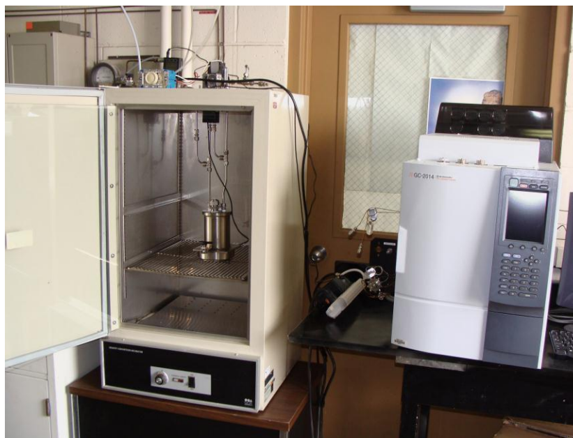
Figure 2-1. Schematic diagram and photos of the experimental setup for VLE measurement
