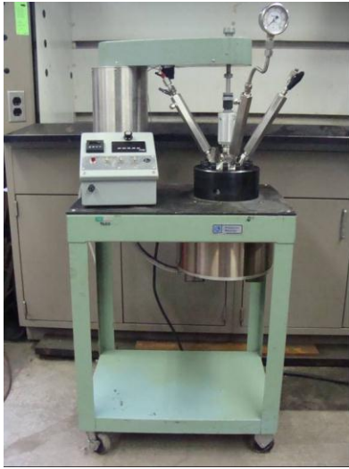
Figure 5-4. Photographs of a Parr autoclave reactor used for PC solution treatment under high-pressure CO 2 gas.
