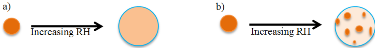
Figure 9 Conceptual overview of the LVA a) and DEMA b) refractive index mixing rules
